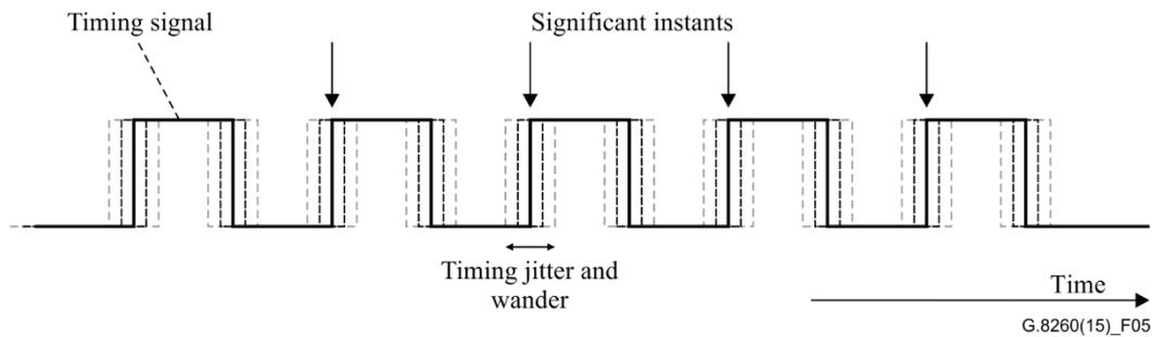
**Figure 5 – Physical layer timing signal**
