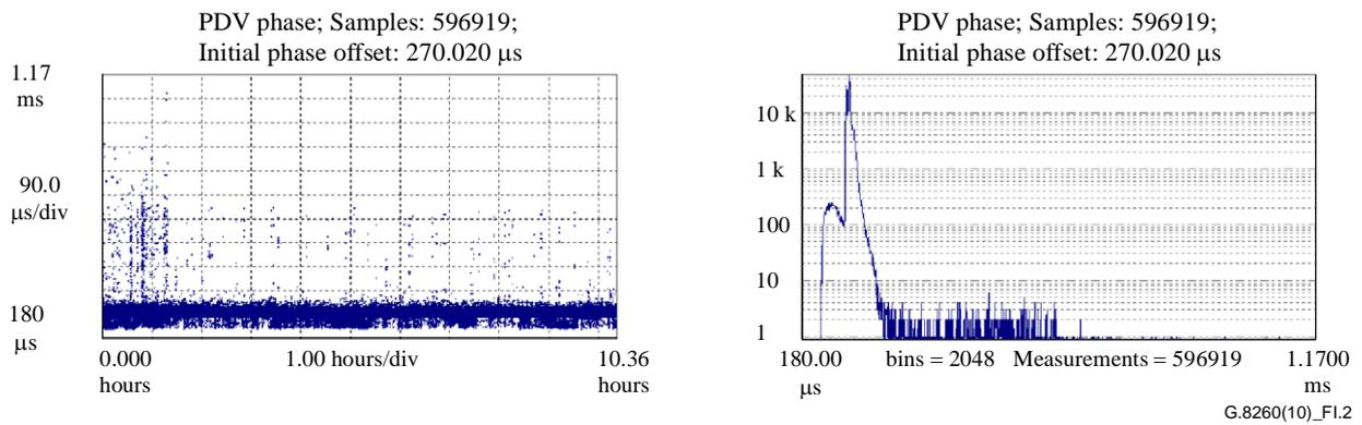
**Figure I.2 – Measured packet delay and corresponding PDV histogram**
