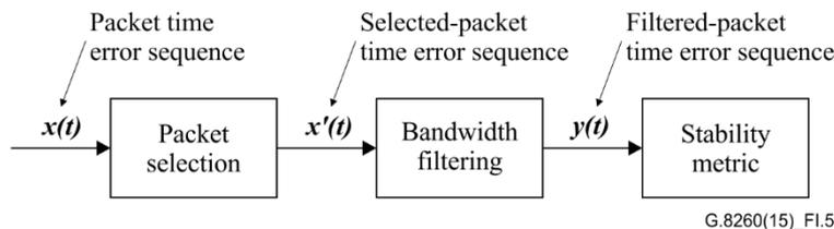
**Figure I.5 – Packet selection and filtering flow**
