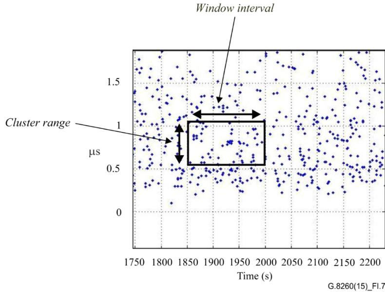
**Figure I.7 – Example of concept of cluster range packet selection**
