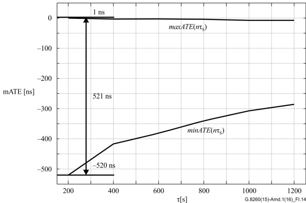
**Figure I.14 – Example of average time error calculation**
