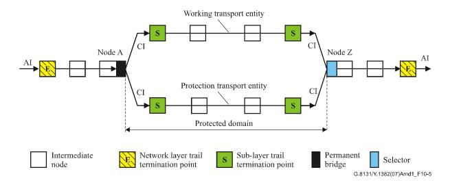
Figure 110-5 – Unidirectional 1+1 SNC/S protection switching architecture
