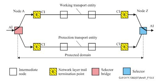
Figure 1<u>10</u>-3 – Bidirectional 1:1 trail protection switching architecture unidirectional representation
