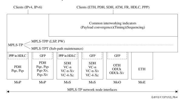
Figure 6-4 – Structure of the MPLS-TP network node interfaces
