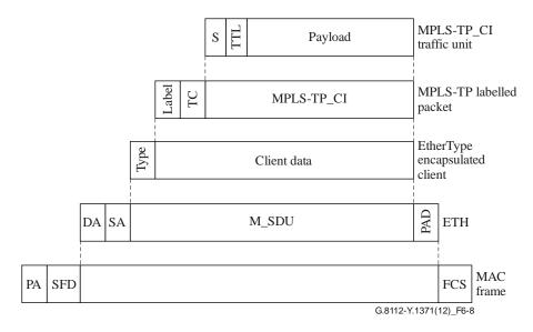
Figure 6-8 – Type encapsulation ETH link frame
