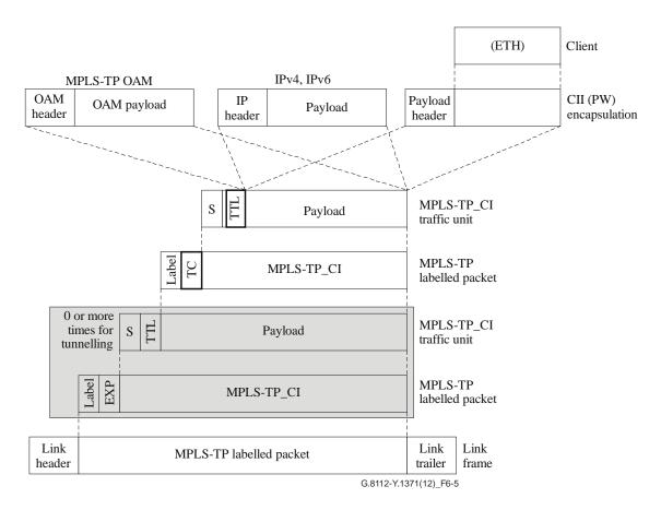
Figure 6-5 – MPLS-TP principle information containment
