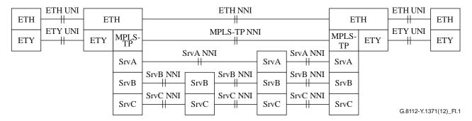
Figure I.1 – Example of layer networks in ETH UNI and MPLS-TP NNI
