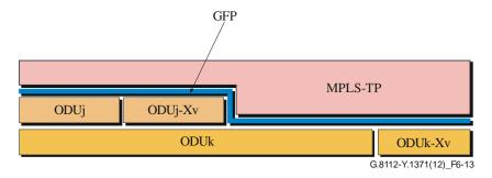
Figure 6-13 – Components of the MPLS-TP over OTH NNI
