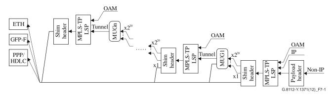
Figure 7-1 – MPLS-TP mapping, multiplexing and segment monitoring
