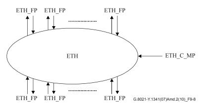
Figure 9-8 – ETH connection function
