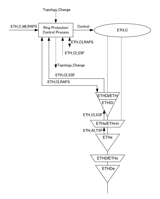
Figure 9-z – Ring protection atomic functions and control process
