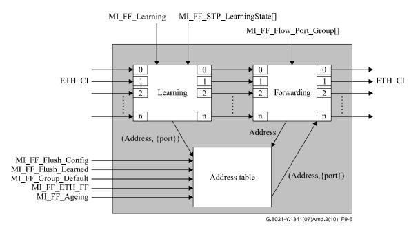
Figure 9-6 – ETH flow forwarding process
