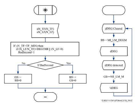
Figure 6-3 – dDEG detection and clearance process
