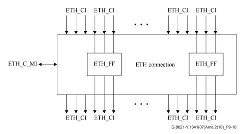
**Figure 9-10 – ETH connection function with ETH\_FF processes**
