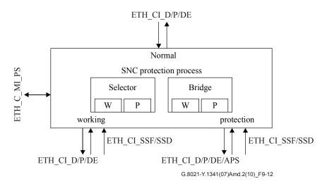
Figure 9-12 – SNC/S protection process
