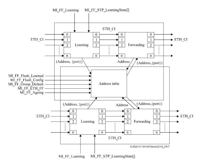
Figure 9-7 – ETH flow forwarding process in SVL mode
