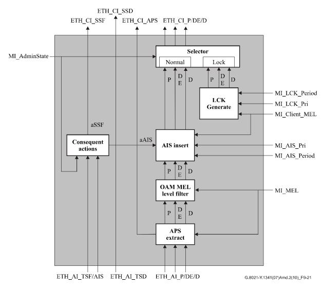
Figure 9-21 – Sink direction ETHx/ETH\_A\_Sk process
