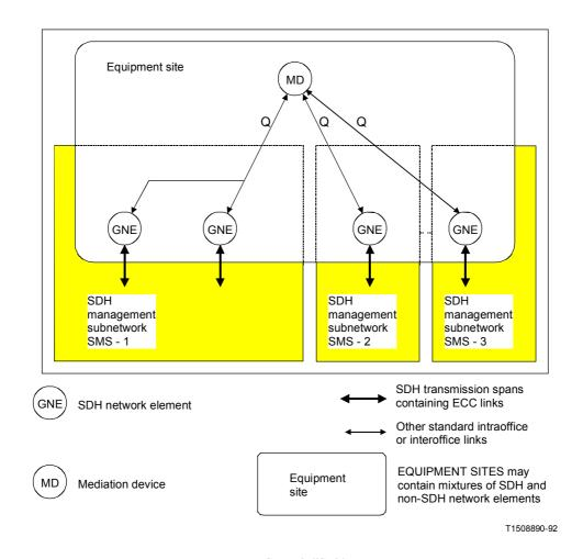
$\label{eq:FIGURE 3-6/G.784} FIGURE \ 3-6/G.784$  SDH ECC topology for sites with mediation devices
