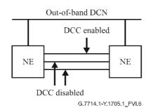
Figure VI.6/G.7714.1/Y.1705.1 – Central Office with DCC enabled on only one link or using an out-of-band DCN
