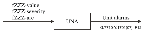
Figure 12 – Unit alarms function
