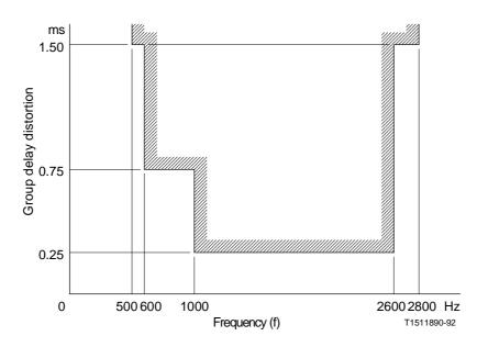
$\label{eq:Group} FIGURE \ 6/G.712 \\ \textbf{Group delay distortion with frequency for analogue-to-analogue channels} \\ \textbf{between 4-wire ports (E4}_{lin} \textbf{ to E4}_{2out} \, )$
