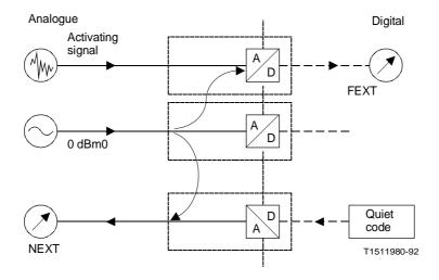
FIGURE 16/G.712 Measurements on 4-wire (E4) ports with analogue test signal between different channels
