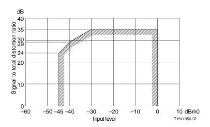
$$\begin{split} & FIGURE~12/G.712\\ \textbf{Signal-to-total distortion ratio as a function of input level}\\ & \textbf{for analogue-to-digital channels}\\ & \textbf{(E4}_{n}~to~T_{out},~T_{in}~to~E4_{out},~E2_{in}~to~T_{out}~and~T_{in}~to~E2_{out}) \end{split}$$
