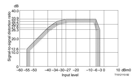
$FIGURE\ A-5/G.712$  Signal-to-total distortion ratio as a function of input level for 4-wire analogue-to-analogue connections (E4 $_{\rm lin}$  to E4 $_{\rm 2out}$ )
