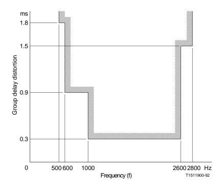
$FIGURE\ 7/G.712$  Group delay distortion with frequency for analogue-to-analogue channels between 2-wire ports (E2 $_{\rm lin}$  to E2 $_{\rm 2out}$ )
