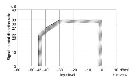
$FIGURE\ 11/G.712$  Signal-to-total distortion ratio as a function of input level for analogue 4-wire to 4-wire and 2-wire to 2-wire channels  $(E4_{in}\ to\ E4_{but}\ and\ E2_{tin}\ to\ E2_{out}\ )$
