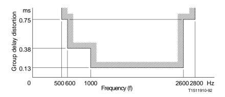
FIGURE~8/G.712 Group delay distortion with frequency for 4-wire analogue-to-digital channels (E4<sub>in</sub> to T<sub>out</sub> or T<sub>in</sub> to E4<sub>out</sub>)
