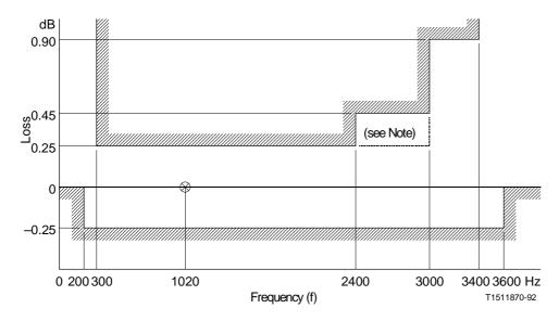
$\it Note-In$  some applications in which several PCM channels may be connected in tandem, it may be necessary to extend the +0.25 dB limit from 2400 Hz to 3000 Hz.
