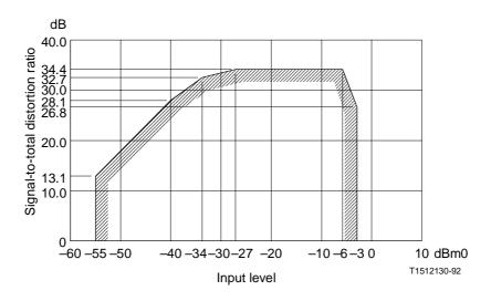
$FIGURE\ A-7/G.712$  Signal-to-total distortion ratio as a function of input level for 4-wire analogue-to-digital encoding side (E4 $_{\rm in}$  to  $T_{\rm out})$
