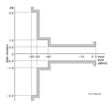
$FIGURE~13/G.712\\ \textbf{Variation of gain with input level for analogue 4-wire to 4-wire and 2-wire to 2-wire channels}\\ (E4_{1in}~to~E4_{2out}~and~E2_{1in}~to~E2_{2out})$
