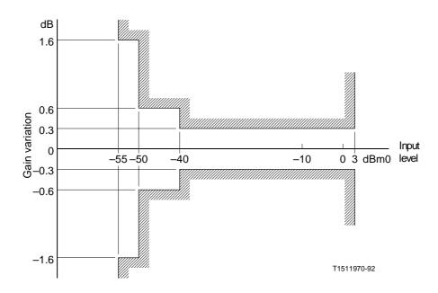
$FIGURE\ 14/G.712$  Variation of gain with input level for analogue-to-digital channels  $(E4_{in}\ to\ T_{out},\ T_{in}\ to\ E4_{out},\ E2_{in}\ to\ T_{out},\ and\ T_{in}\ to\ E2_{out})$
