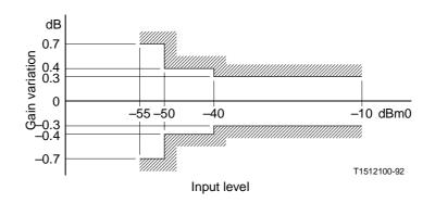
$FIGURE\ A-4/G.712$  Variation of gain with input level for analogue-to-digital channels (E4 $_{\rm in}$  to T $_{\rm out}$ , T $_{\rm in}$  to E4 $_{\rm out}$ , E2 $_{\rm in}$  to T $_{\rm out}$ , or T $_{\rm in}$  to E2 $_{\rm out}$ )
