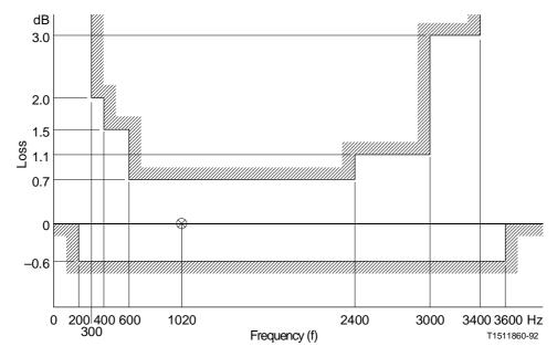
Note -Some Administration apply a limit of 1 dB maximum loss for the frequency range 300 Hz to 3000 Hz
