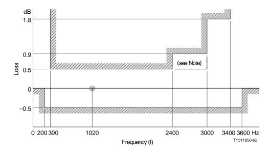
Note- In some applications in which several PCM channels may be connected in tandem, it may be necessary to extend the +0.5 dB limit from 2400 Hz to 3000 Hz.
