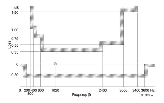
$\it Note-Some$  Administrations apply a limit of 0.5 dB maximum loss for the frequency range 300 Hz to 3000 Hz.
