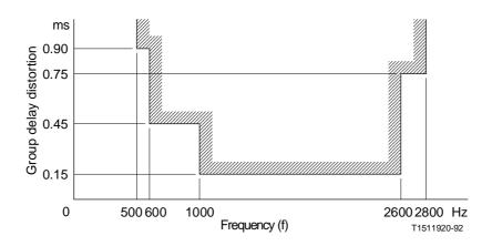
FIGURE~9/G.712 Group delay distortion with frequency for 2-wire analogue-to-digital channels (E2<sub>in</sub> to T<sub>out</sub> or T<sub>in</sub> to E2<sub>out</sub>)
