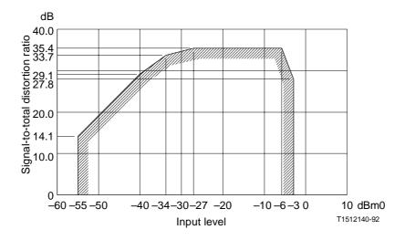
$\it Note - The values in the mask include the distortion power of an ideal encoder.$
