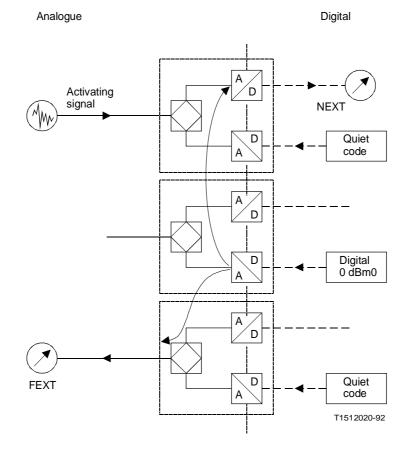
FIGURE 20/G.712 Measurements on 2-wire (E2) ports with digital test signal between different channels
