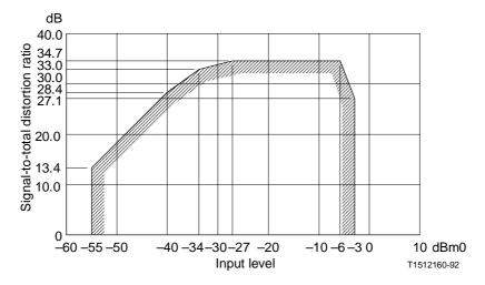
${\it Note}-{\it The \, values \, in \, the \, mask \, include \, the \, distortion \, power \, of \, an \, ideal \, encoder.}$
