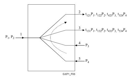
Figure 3/G.671 – Example of bidirectional (near-end) isolation
