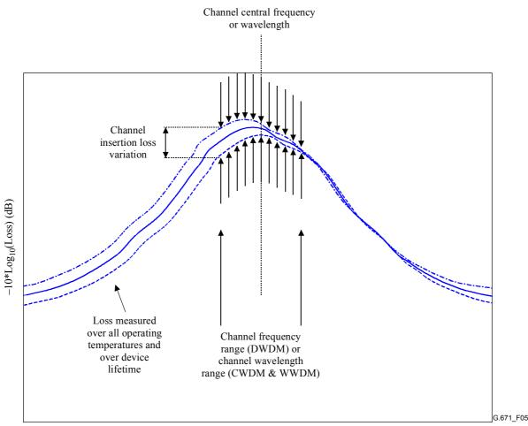
Optical frequency (THz) for DWDM or wavelength (nm) for CWDM & WWDM
