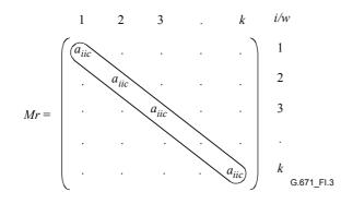
Figure I.3/G.671 – Matrix Mr for a  $k\lambda$ -MUX
