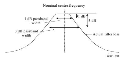
Figure 1/G.671 – Illustration of 1 dB and 3 dB passband width
