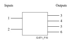
Figure 10/G.671 – An example of the port assignments for the transfer matrix
