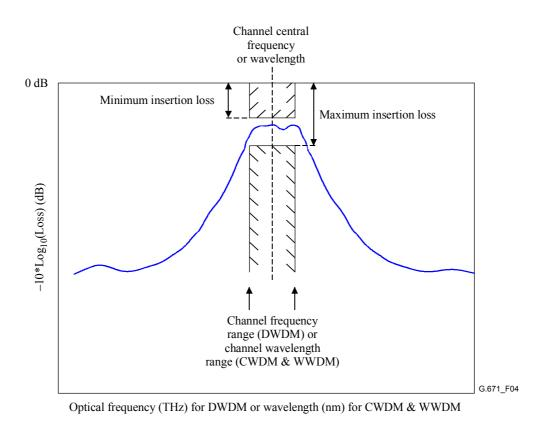
Figure 4/G.671 – Illustration of maximum and minimum insertion loss of a WDM device
