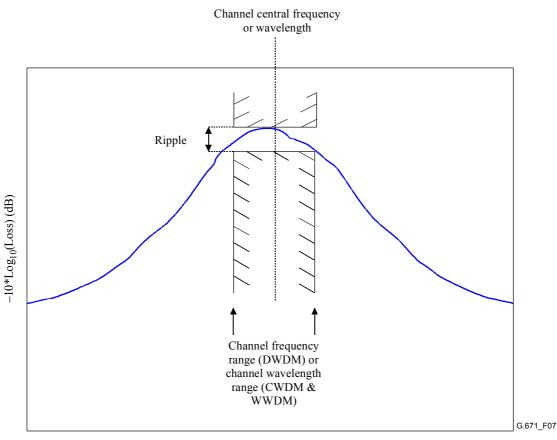
Optical frenquency (THz) for DWDM or wavelength (nm) for CWDM & WWDM
