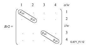
Figure I.12/G.671 – Matrix Br2 for a 4λ-DMUX/MUX2
