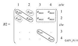
Figure I.11/G.671 – Matrix B2 for a 4λ-DMUX/MUX2
