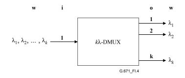
Figure I.4/G.671 –  $k\lambda$ -DMUX port numbering
