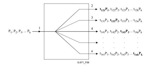
Figure 9/G.671 – Example of WDM demultiplexer device
