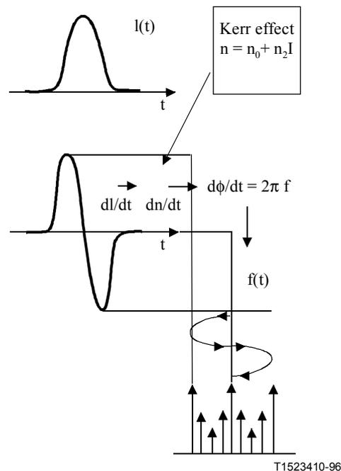
**Figure II.3-1 – Spectral broadening mechanism due to self-phase modulation**
