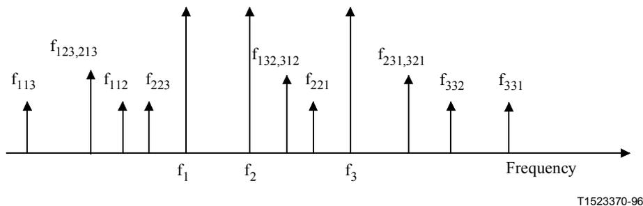
**Figure II.3-4 – Mixing products generated due to four-wave mixing of three signals**
