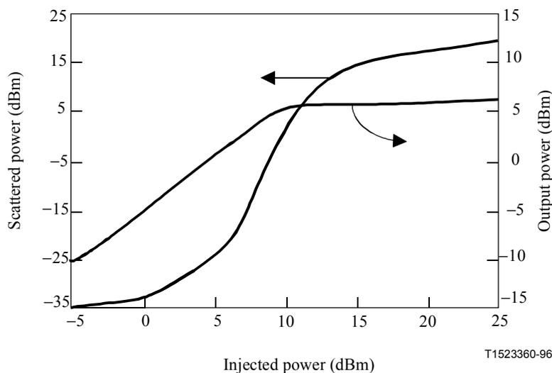
**Figure II.3-6 – Stimulated Brillouin scattering effect for narrow-band source**
