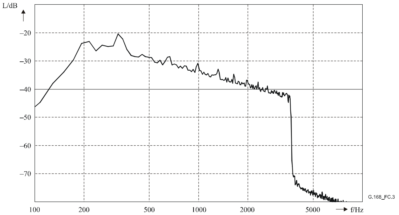
Figure C.3/G.168 – Power density spectrum of the bandlimited CSS (single talk signal, analysis window: Hanning)
