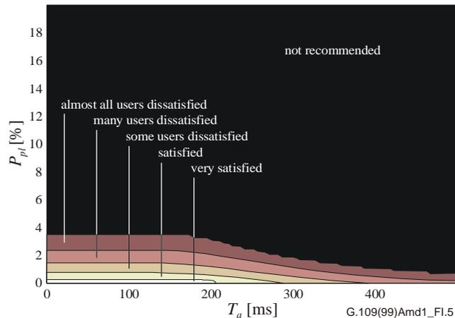
**Figure I.5 – Quality contours calculated for G.711 encoding scheme (random packet loss) without PLC**
