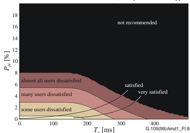
**Figure I.8 – Quality contours calculated for G.729A encoding scheme (bursty packet loss) with PLC**
