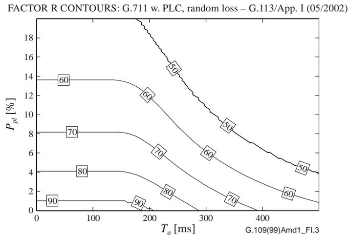
**Figure I.3 – Contours of rating factor  $R$  calculated for G.711 encoding scheme (random packet loss, PLC)**
