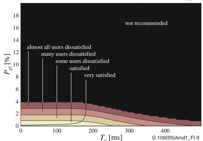
**Figure I.9 – Quality contours calculated for G.729E encoding scheme (bursty packet loss) with PLC**
