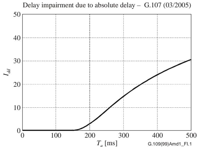
Figure I.1 – Delay impairment  $I_{dd}$  as a function of absolute transmission delay  $T_a$
