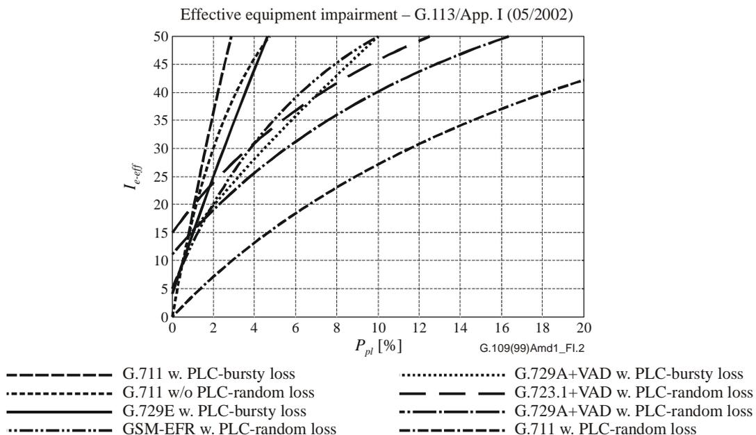
Figure I.2 – Effective Equipment Impairment  $I_{e-eff}$  as a function of packet loss  $P_{pl}$
