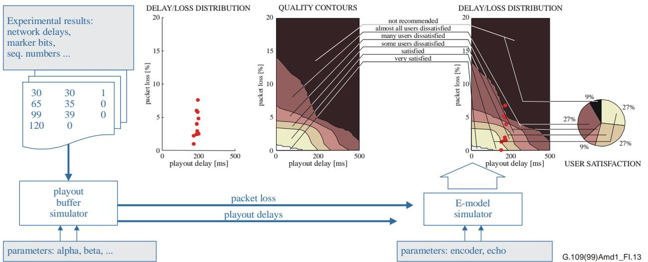
**Figure I.13 – Evaluating playout buffer algorithms with the use of the proposed method**
