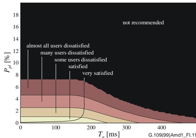
**Figure I.11 – Quality contours calculated for GSM 06.60 (EFR) encoding scheme (random packet loss) with PLC**
