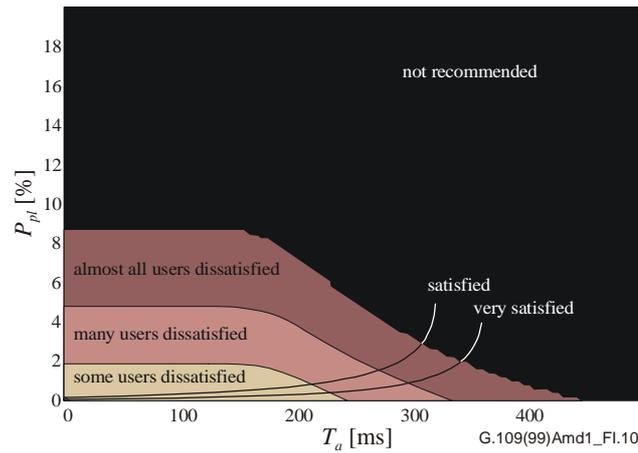
**Figure I.10 – Quality contours calculated for G.723.1 encoding scheme (random packet loss) with PLC**
