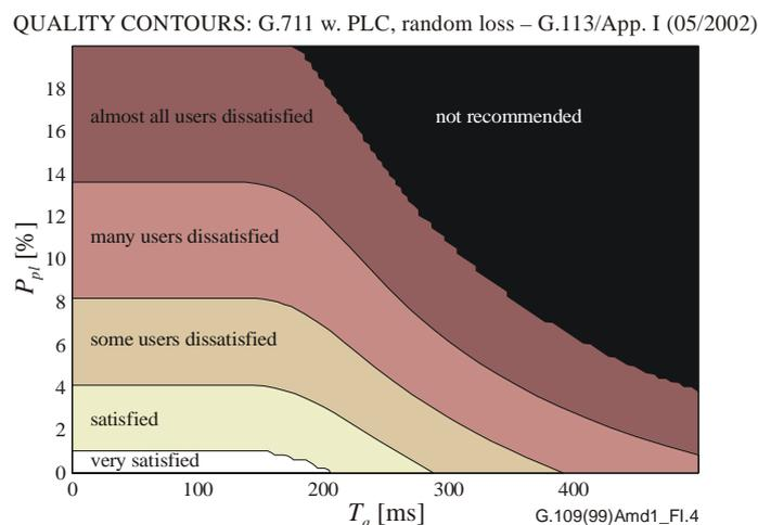
**Figure I.4 – Contours of user satisfaction (contours of speech transmission quality) for G.711 encoding scheme (random packet loss, PLC)**
