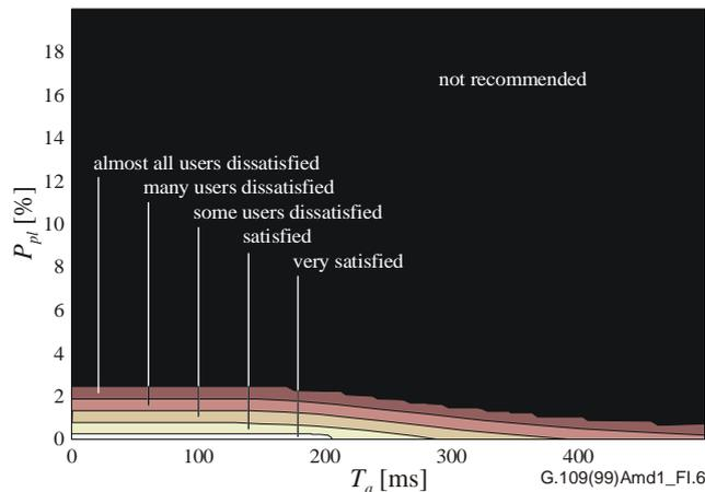
**Figure I.6 – Quality contours calculated for G.711 encoding scheme (bursty packet loss) with PLC**
