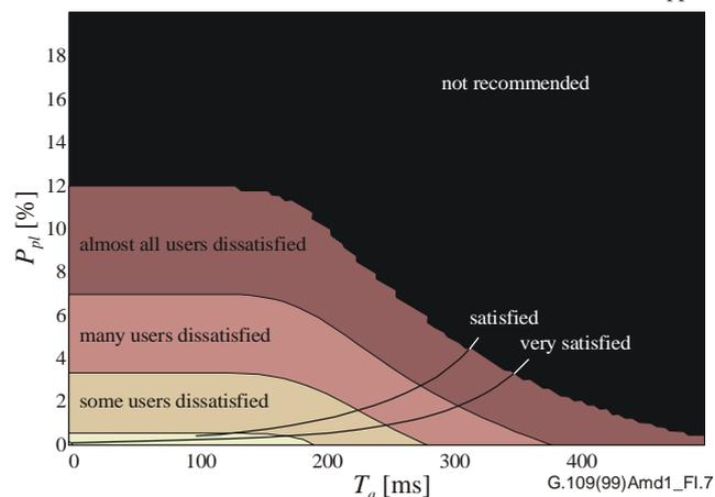
**Figure I.7 – Quality contours calculated for G.729A encoding scheme (random packet loss) with PLC**
