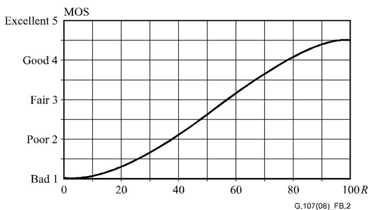
**Figure B.2 – MOS<sub>CQE</sub> as function of rating factor *R***
