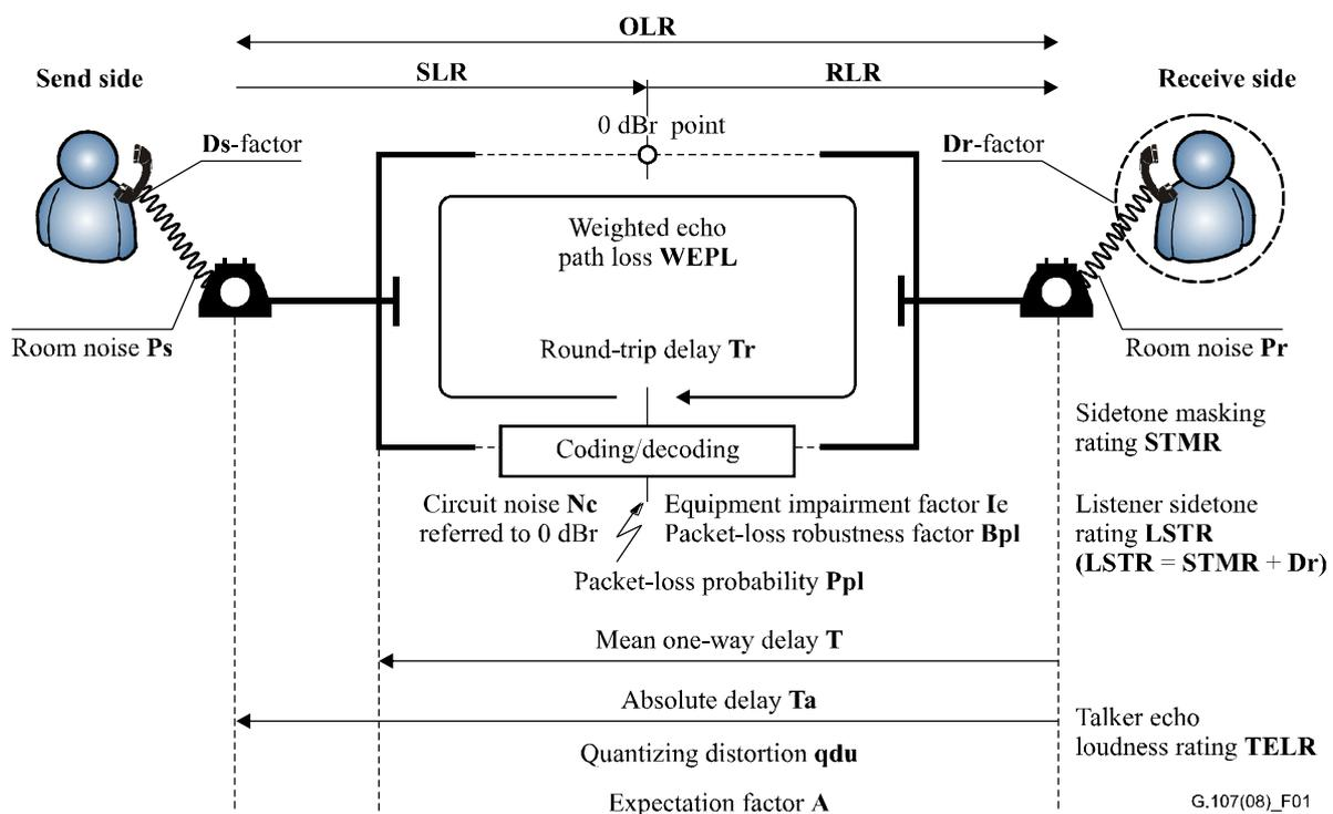
Figure 1 – Reference connection of the E-model
