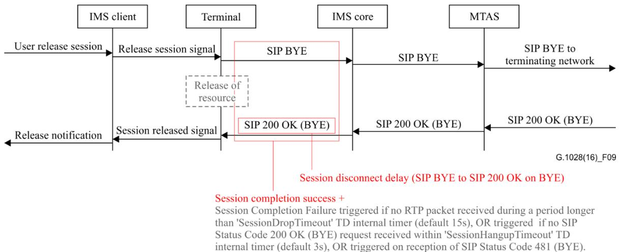
**Figure 9 – VoLTE session completion measurement flow**
