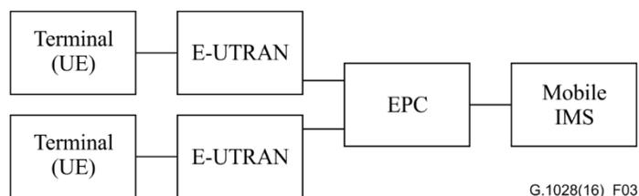
**Figure 3 – Hypothetical reference model for an LTE-LTE communication on the same network**
