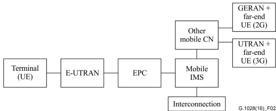
**Figure 2 – Simplified architecture of VoLTE services**
