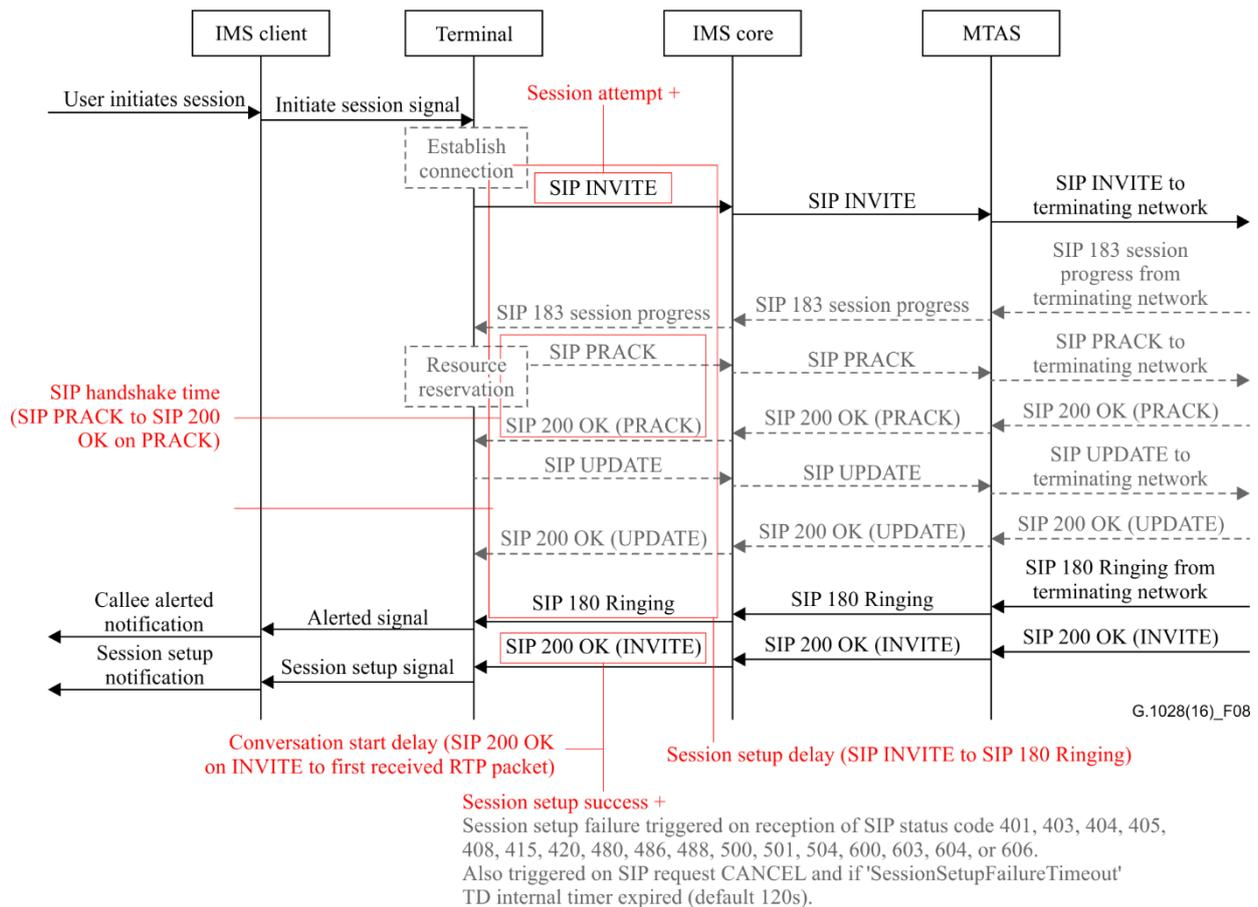
**Figure 8 – VoLTE session set-up measurement flow**
