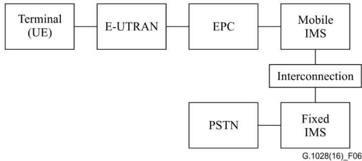
**Figure 6 – Hypothetical reference model for an LTE-PSTN communication**
