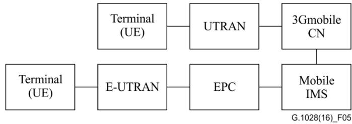
**Figure 5 – Hypothetical reference model for an LTE-3G communication**
