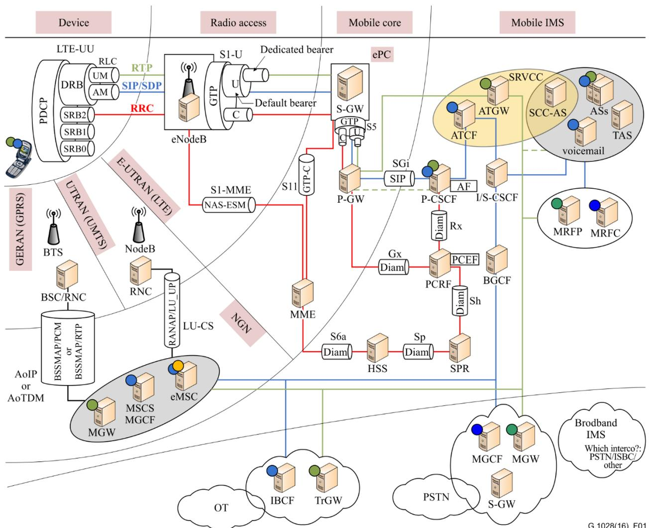
**Figure 1 – Overall architecture of VoLTE services**
