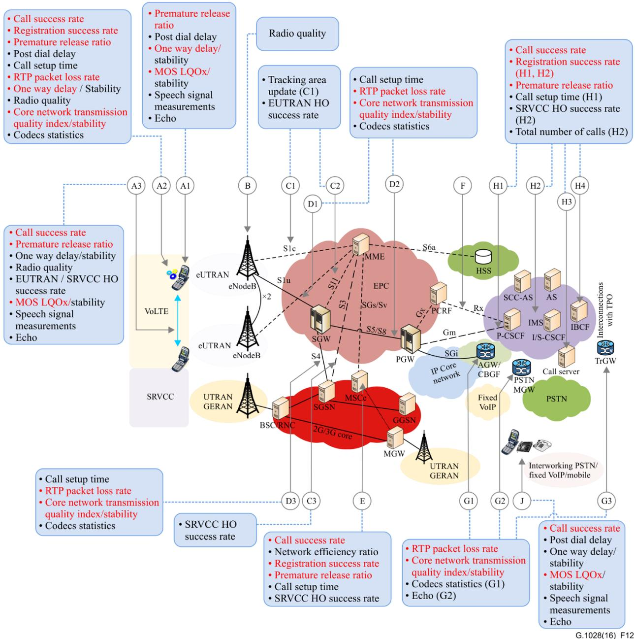
Figure 12 – VoLTE QoS measurement points – monitoring
