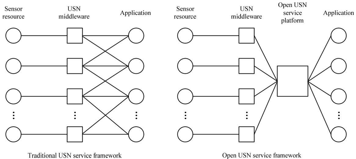
**Figure 6-1 – Traditional USN service framework and open USN service framework**
