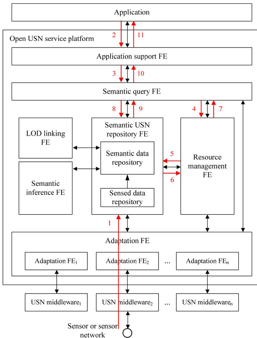
**Figure I.2 – Information flow of accessing sensed data/semantic data from Semantic USN repository FE**
