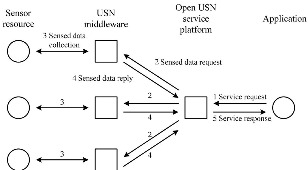
**Figure 6-2 – Heterogeneous USN middleware access through the open USN service platform**
