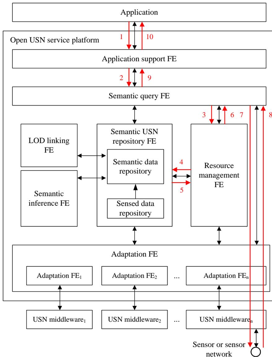
**Figure I.3 – Information flow of accessing sensed data from USN resources**
