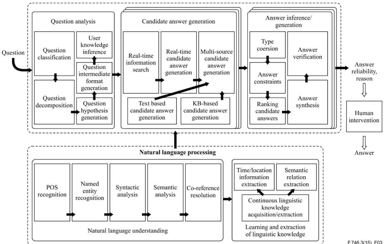
Figure 3 – Logical functional block diagram of an IQAS
