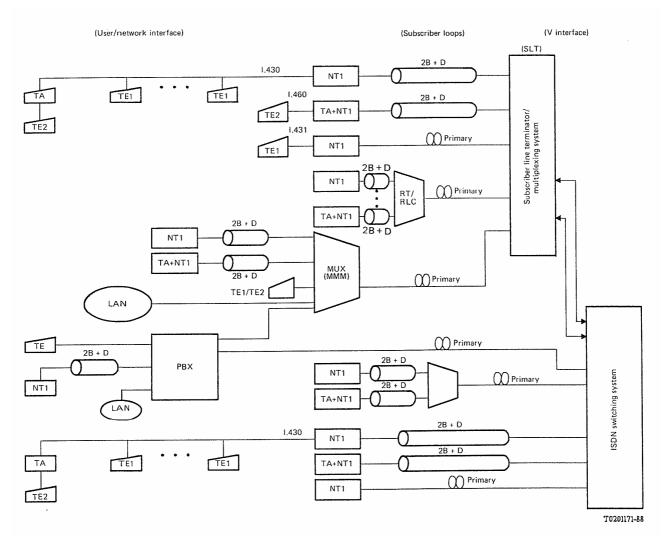
Note - The equipments and channels shown in this diagram are defined in Recommendations I.411 and I.412.
