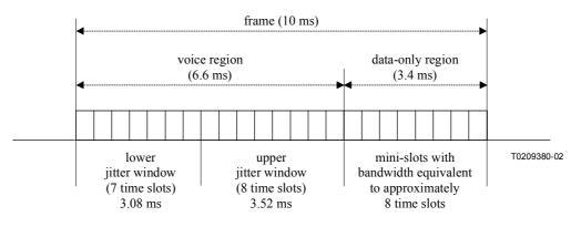
Figure II.1/E.681 – Example frame structure with two jitter windows
