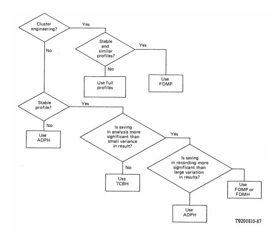
FIGURE 2/E.500 Flow chart for choosing the measurement method
