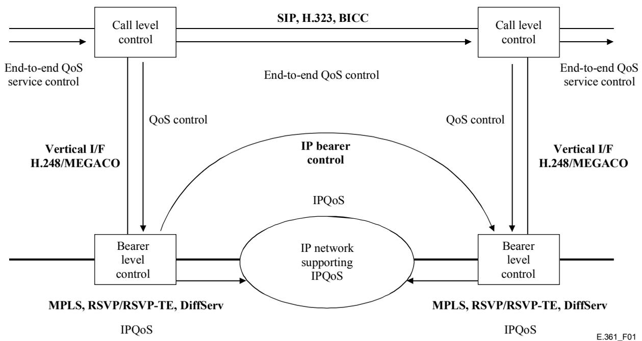
**Figure 1/E.361 – Framework for end-to-end QoS Control in IP-based networks**
