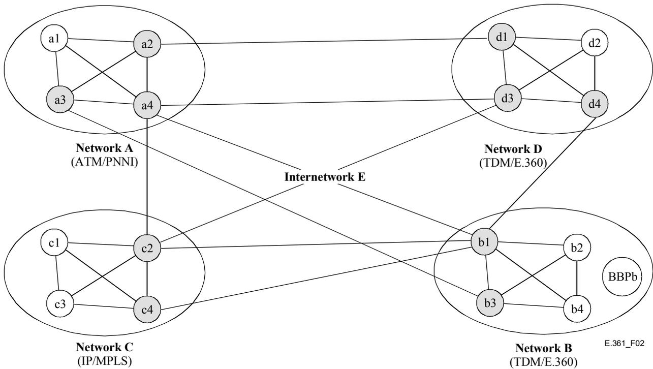
**Figure 2/E.361 – Example of an internetwork QoS routing and signalling scenario**
