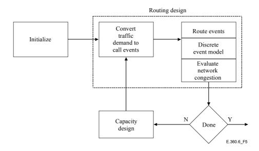
Figure 5/E.360.6 – Discrete Event Flow Optimization (DEFO) model
