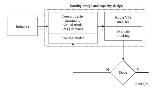
Figure 8/E.360.6 – Virtual Trunking Flow Optimization (VTFO) model
