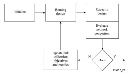
Figure 7/E.360.6 – Traffic Load Flow Optimization (TLFO) model
