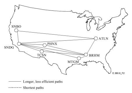
Figure 2/E.360.6 – Shortest path routing
