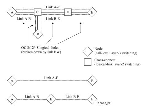
Figure 11/E.360.6 – Mesh logical network topology with logical-link layer-2 switching and call-level layer-3 switching
