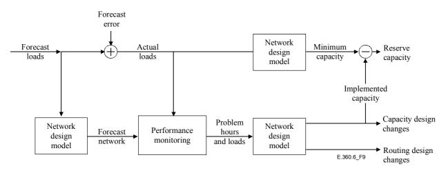
Figure 9/E.360.6 – Design model illustrating forecast error and reserve capacity trade-off
