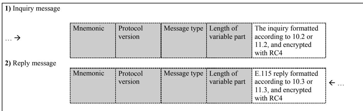
The fixed-length header contains four fields and is used by the DA applications to determine the beginning of the message and the size of the variable part to be processed.
