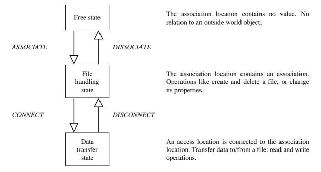
The model assumes that objects, in implementations often referred to as datasets, files or devices, exist in the outside world, i.e. the external environment of a CHILL program. Such an outside world object is called a file in the model. A file can be a physical device, a communication line or just a file in a file management system; in general, a file is an object that can produce and/or consume data.
