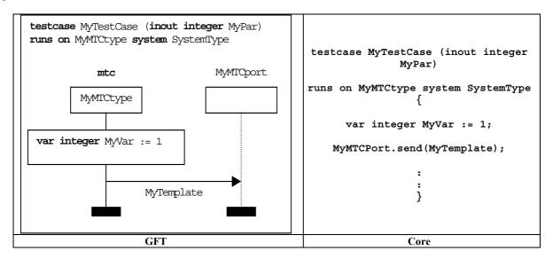
Figure 10/Z.142 - Principle shape of a GFT test case diagram and corresponding core language
