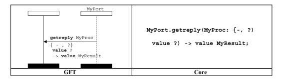
Figure 77/Z.142 – Getreply operation with inline template (outside a call symbol)
