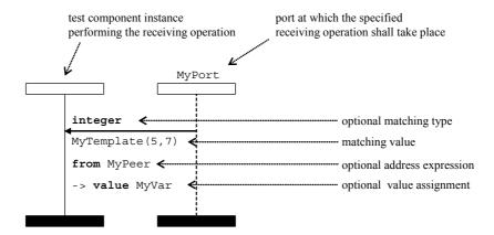
Figure 50/Z.142 – General format of receiving operations with address and value assignment
