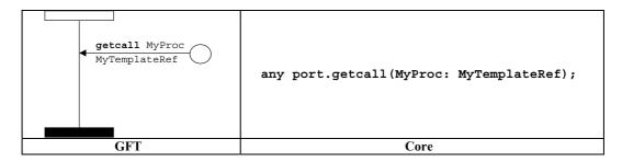
Figure 71/Z.142 – Getcall on any port operation with template reference
