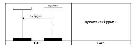
Figure 60/Z.142 - Trigger on any message operation
