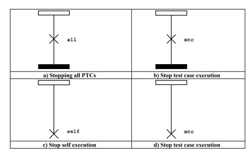
Figure 47/Z.142 – Special usages of the stop test component operation
