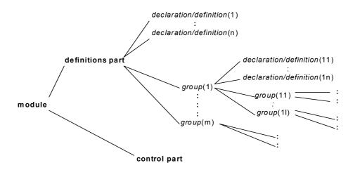
Figure 6/Z.142 – Structure of TTCN-3 modules
