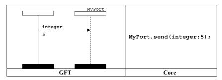
Figure 53/Z.142 - Send operation with inline template
