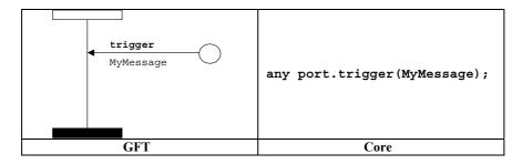
Figure 61/Z.142 - Trigger on any port operation
