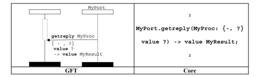
Figure 75/Z.142 – Getreply operation with inline template (within a call symbol)
