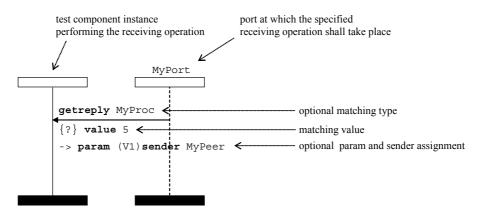
Figure 51/Z.142 – General format of receiving operations with param and sender assignment
