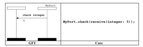
Figure 93/Z.142 – Check a receive with inline template
