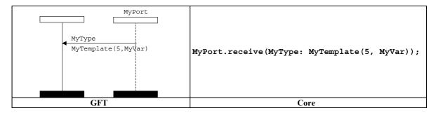
Figure 54/Z.142 – Receive operation with template reference
