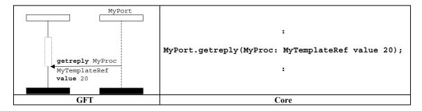
Figure 74/Z.142 – Getreply operation with template reference (within a call symbol)
