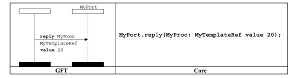
Figure 72/Z.142 – Reply operation with template reference
