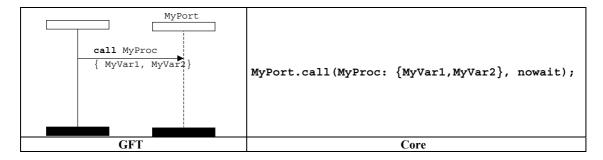
Figure 67/Z.142 – Non-blocking call operation with inline template
