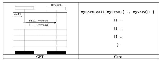
Figure 63/Z.142 – Blocking call operation with inline template
