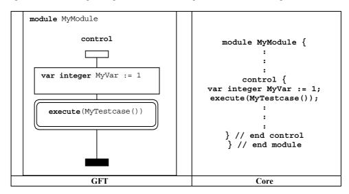
Figure 9/Z.142 – Principle shape of a GFT control diagram and corresponding core language
