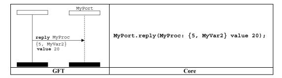
Figure 73/Z.142 – Reply operation with inline template
