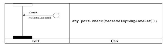
Figure 97/Z.142 - Check a receive on any port
