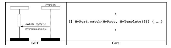
Figure 84/Z.142 – Catch operation with template reference (within a call symbol)
