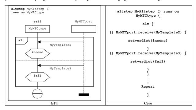
Figure 12/Z.142 - Principle shape of a GFT altstep diagram and corresponding core language
