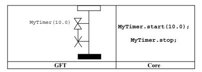
Figure 104/Z.142 – Connected start and stop timer symbols
