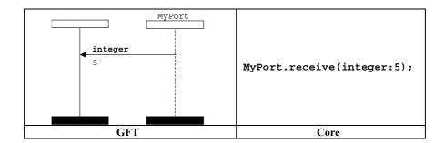
Figure 55/Z.142 – Receive operation with inline template
