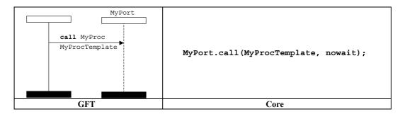
Figure 66/Z.142 - Non-blocking call operation with template reference
