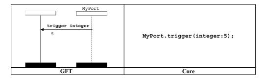
Figure 59/Z.142 – Trigger operation with inline template
