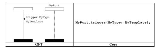
Figure 58/Z.142 – Trigger operation with template reference
