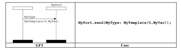
Figure 52/Z.142 – Send operation with template reference
