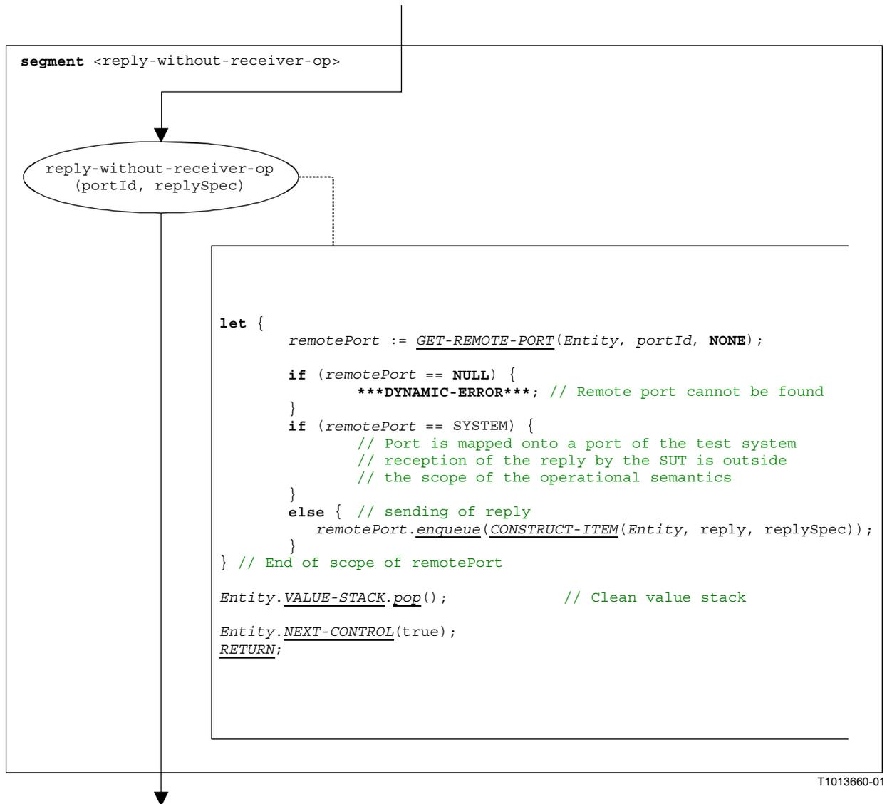
Figure B.98/Z.140 – Flow graph segment <reply-without-receiver-op>
