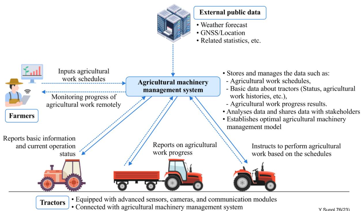
**Figure 5 – Process flow diagram of the connected agricultural tractor**
