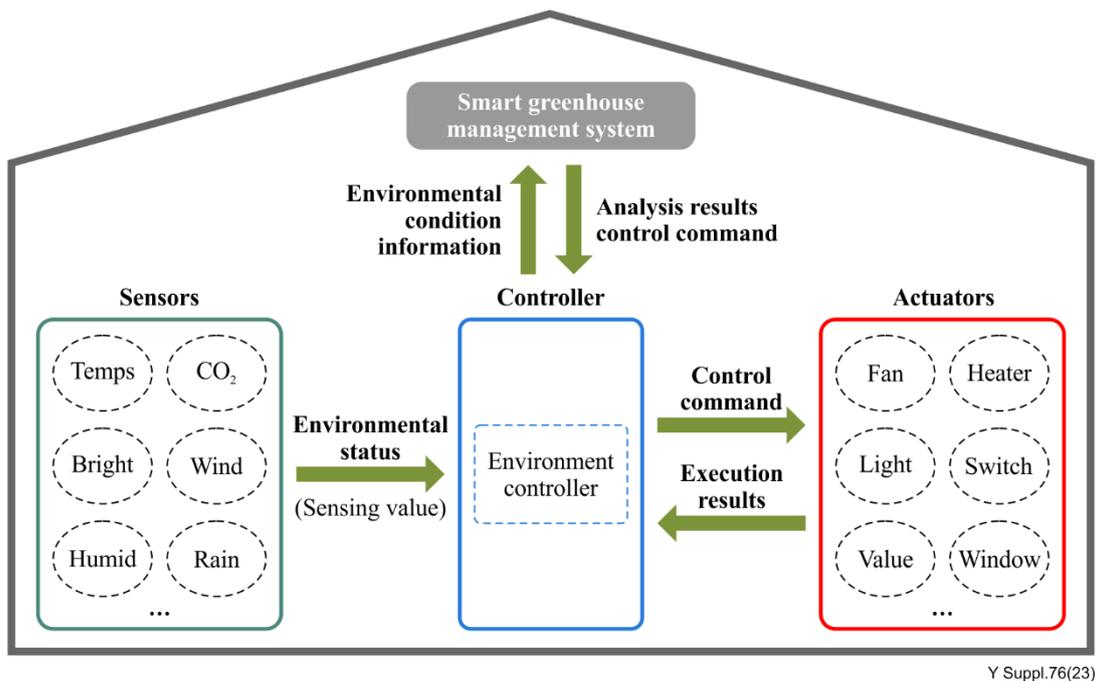
**Figure 1 – Process flow diagram of the smart greenhouse**
