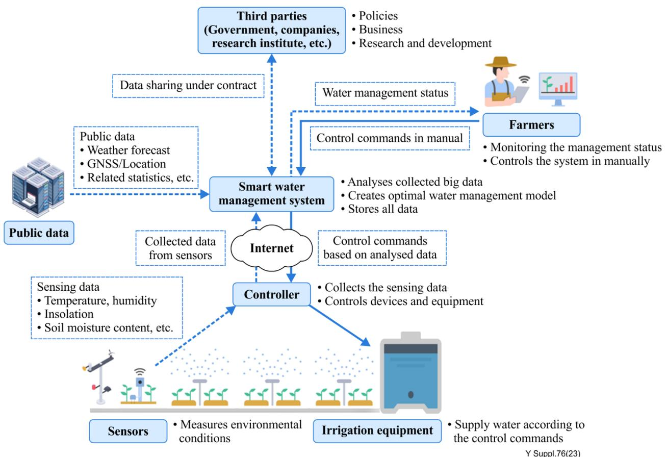
**Figure 3 – Process flow diagram of smart water management service**
