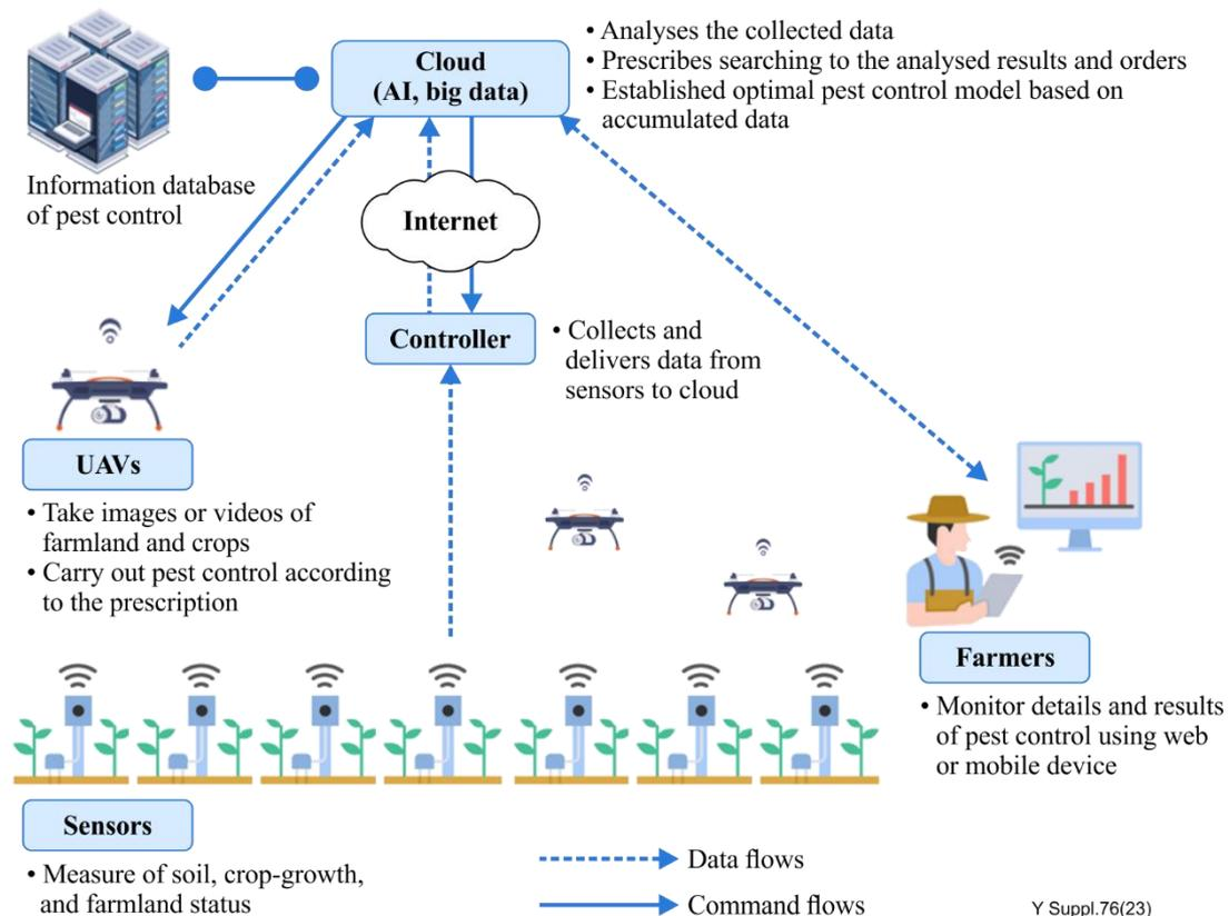
**Figure 4 – Process flow diagram of pest control using UAVs**
