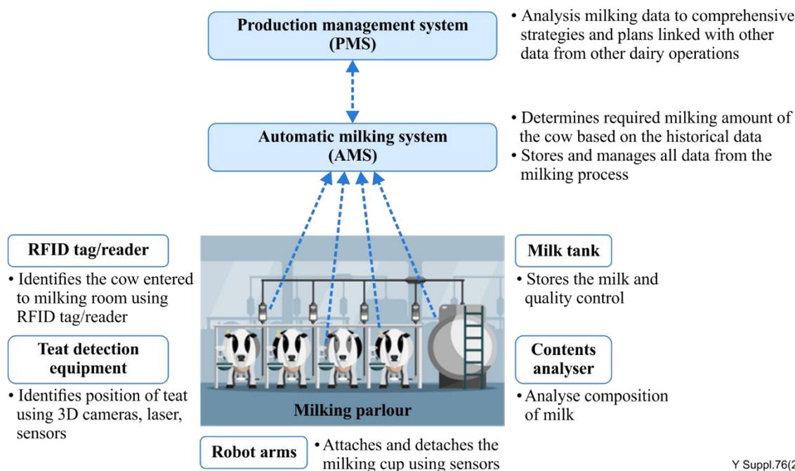
**Figure 6 – Process flow diagram of the AMS in dairy farm**
