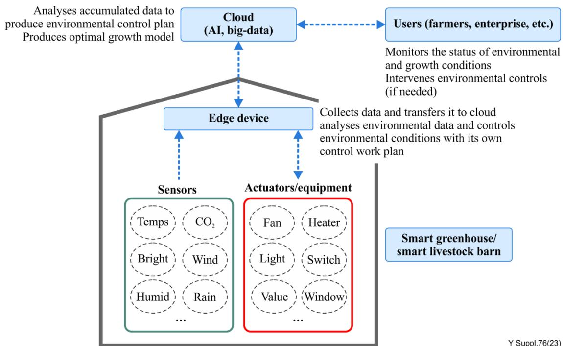
**Figure 2 – Process flow diagram of a smart greenhouse with cloud and edge support**
