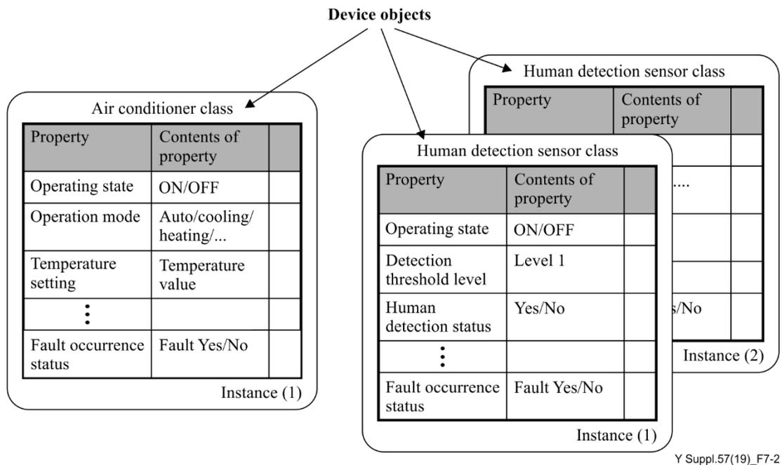
**Figure 7-2 – Device object example**
