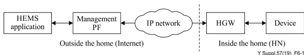
**Figure 6-1 – HEMS based on HN service architecture**
