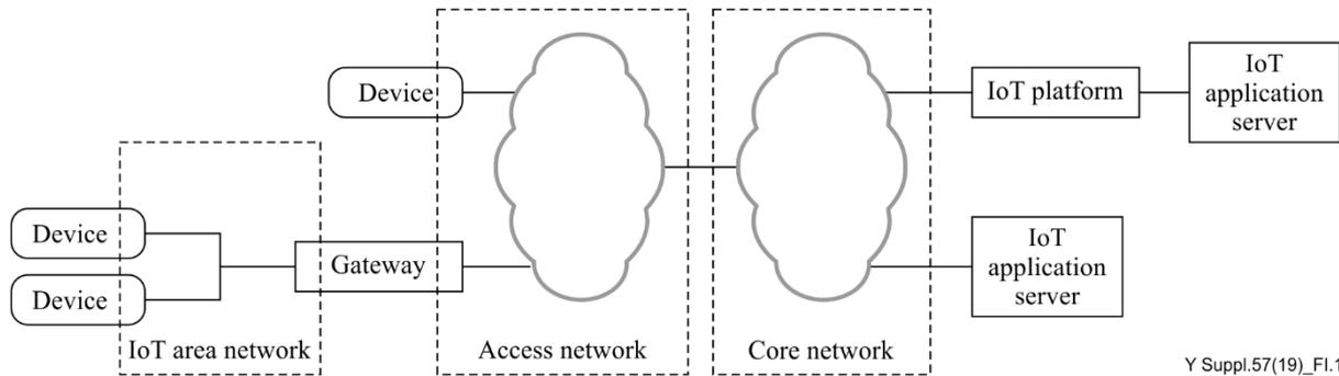
**Figure I.1 – Basic model of the network for the IoT**
