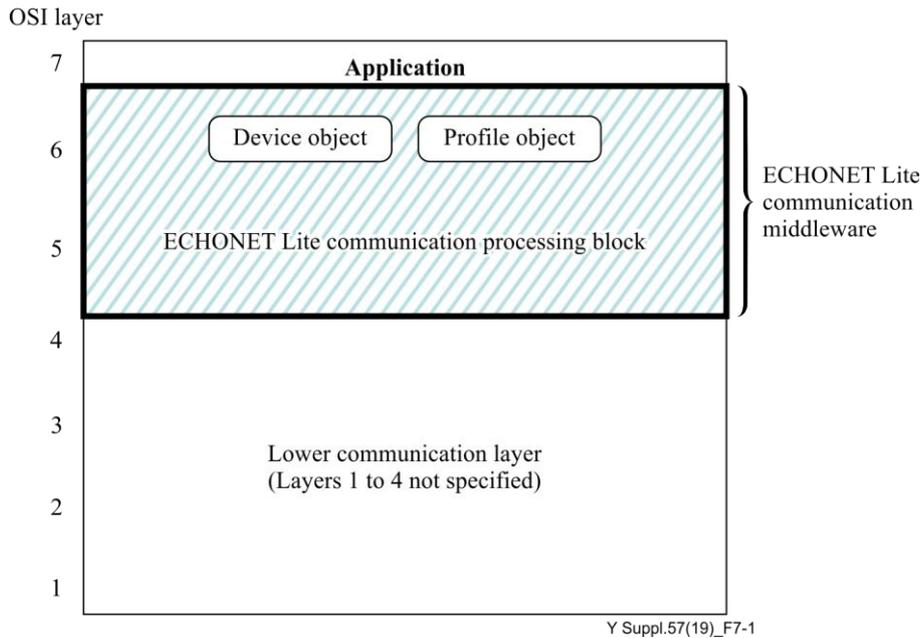
**Figure 7-1 – ECHONET Lite communication layer configuration**
