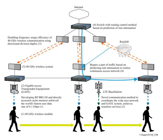
Figure 8 – Schematic overview of proposed wireless network
