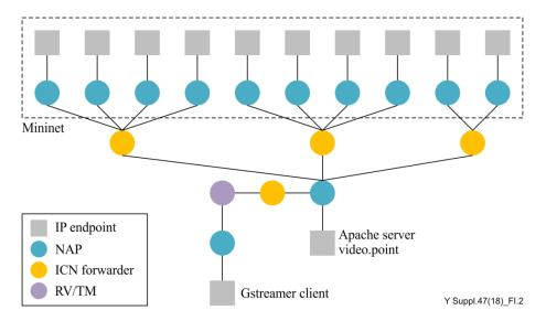
Figure I.2 – Test-bed topology with 10 emulated clients
