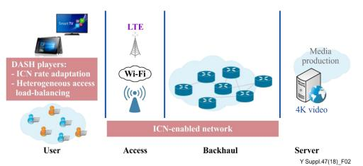
Figure 2 – ICN enhanced mobile video service PoC architecture
