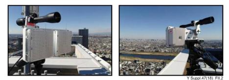
Figure II.2 – Photographs of the 40 GHz wireless system using DDD
