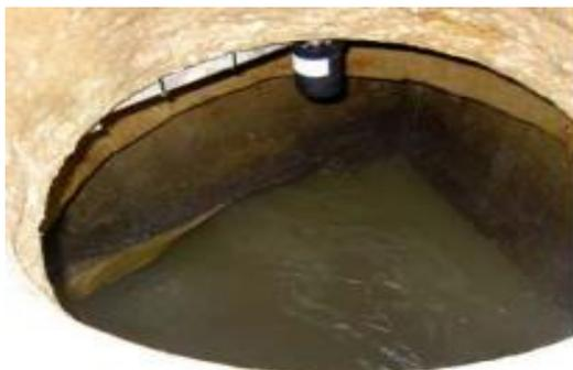
**Figure 18 – SmartScan 50 non-contact gauging device equipped with sensors**
