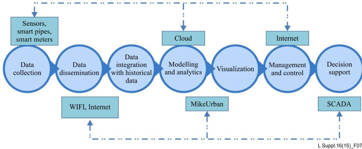
**Figure 7 – Schematic representation of smart water management technologies and tools**
