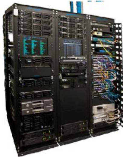
Figure 12 – Rack mounted servers
