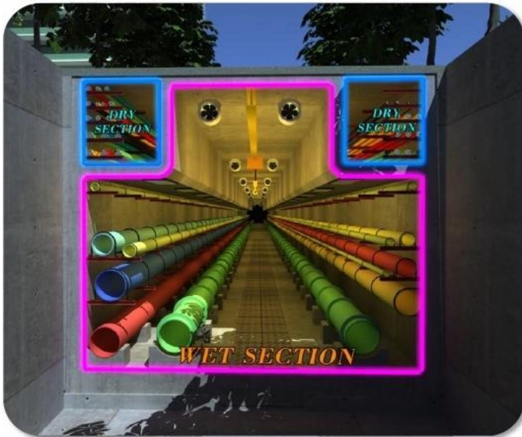
**Figure 10 – Utility tunnel, showing wet and dry sections**
