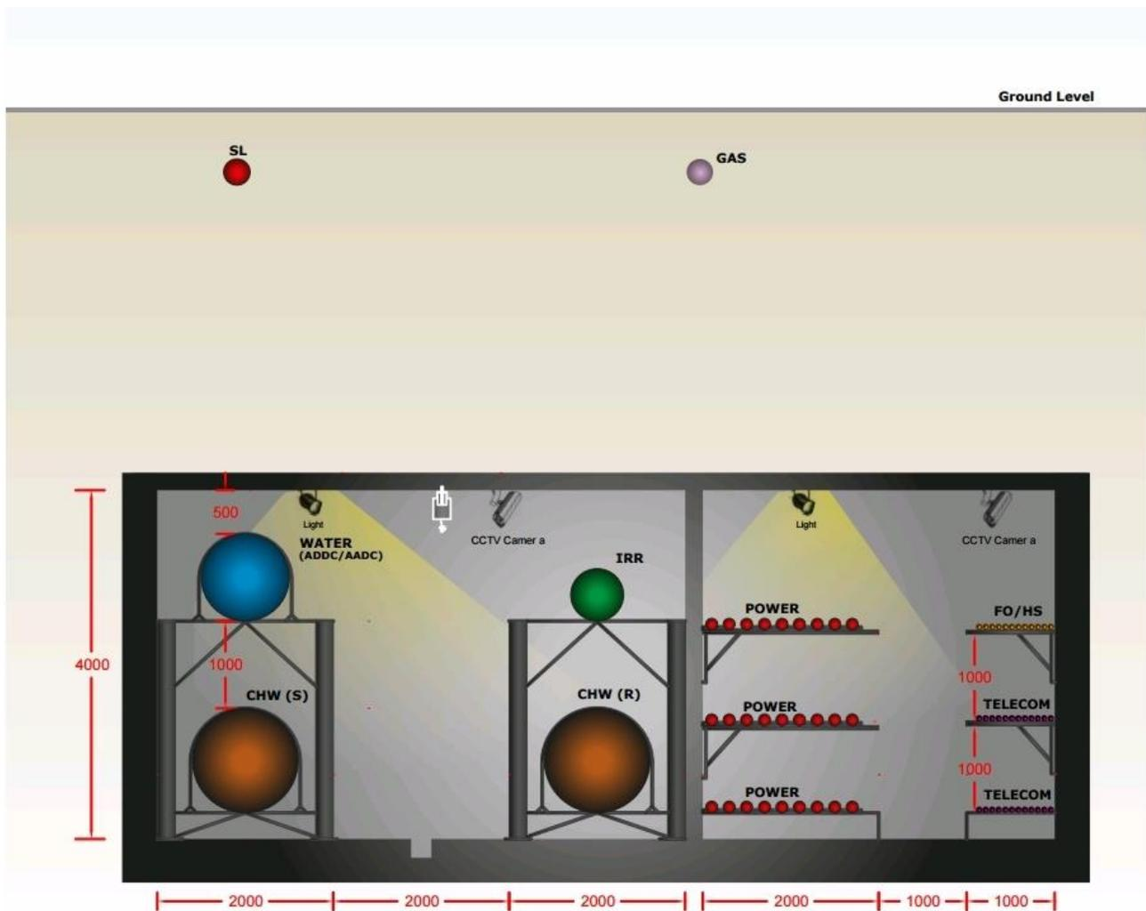
**Figure 9 – Typical arrangement of a utility tunnel**
