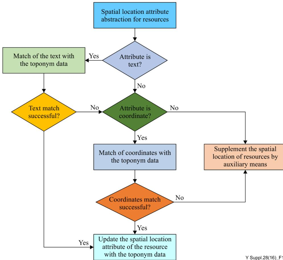
**Figure 16 – Technical workflow of matching resources up with the toponym database in the integrated management for smart sustainable cities**
