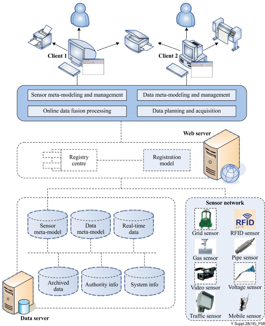
Figure 8 – Architecture of the observation web technology used in smart sustainable cities
