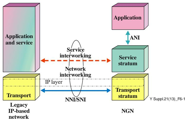
**Figure 6-1 – Interworking model between an NGN and a legacy IP-based network [ITU-T Y.2011]**
