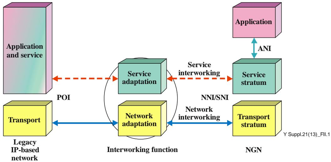
**Figure II.1 – Interworking function between legacy IP-based network and NGN**
