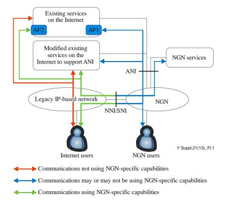
Figure I.1 – An example of interworking between legacy IP-based network and NGN
