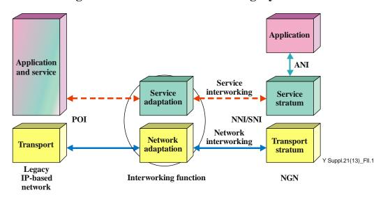
Figure II.1 – Interworking function between legacy IP-based network and NGN
