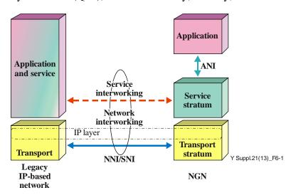
Figure 6-1 – Interworking model between an NGN and a legacy IP-based network [ITU-T Y.2011]
