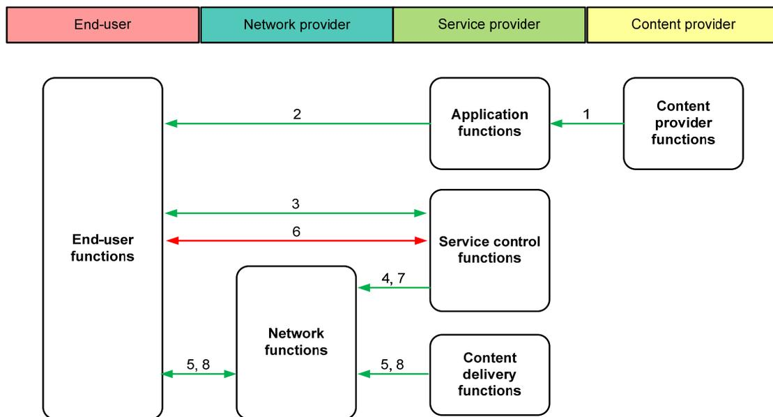
**Figure 8-4 – Use case of n-screen service with service mobility**
