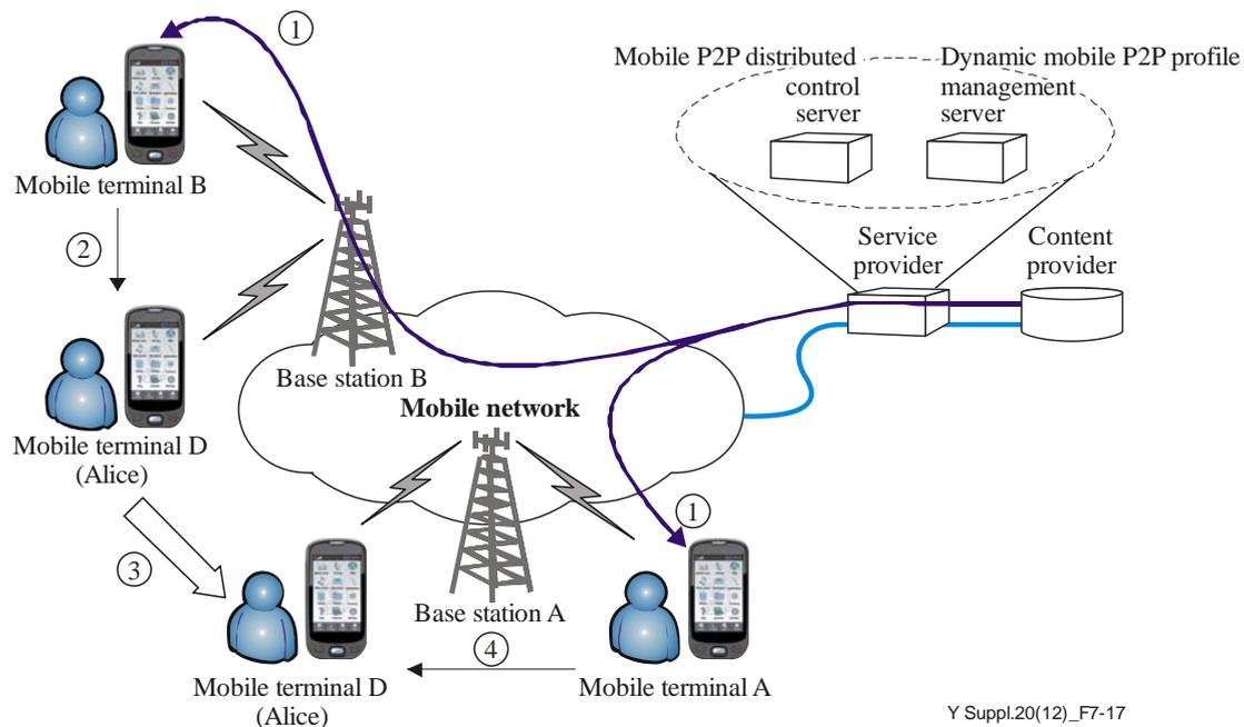
**Figure 7-17 – P2P-based mobile IPTV service**
