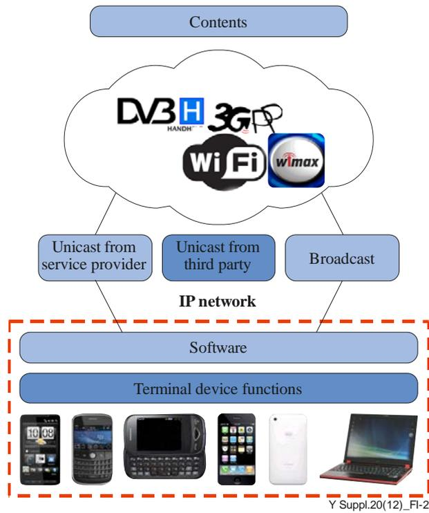
**Figure I.2 – IPTV services based on IP**
