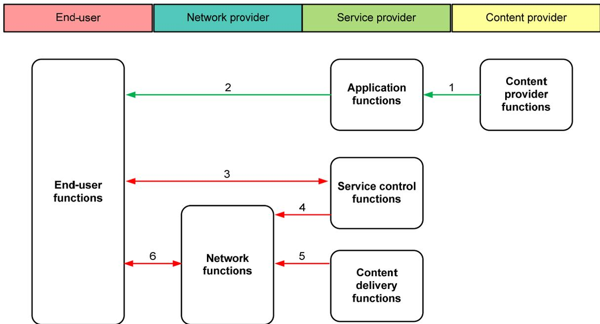
**Figure 8-2 – Use case of n-screen service with contents sharing**
