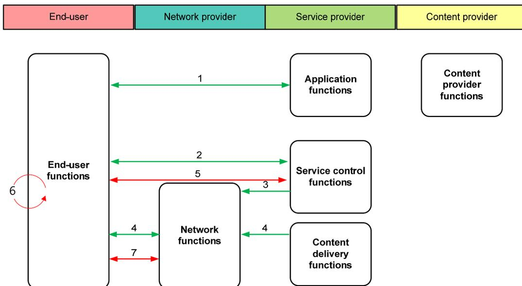
**Figure II.5 – Use case of mobile IPTV service with cost effective peering**
