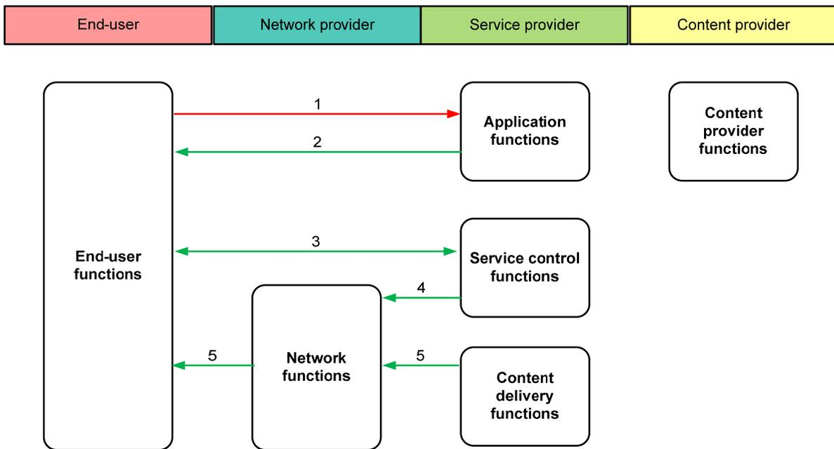
**Figure 7-20 – Use case of UCC delivery over mobile networks**
