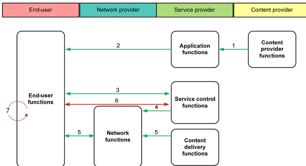
**Figure 7-18 – Use case of P2P-based IPTV content delivery**
