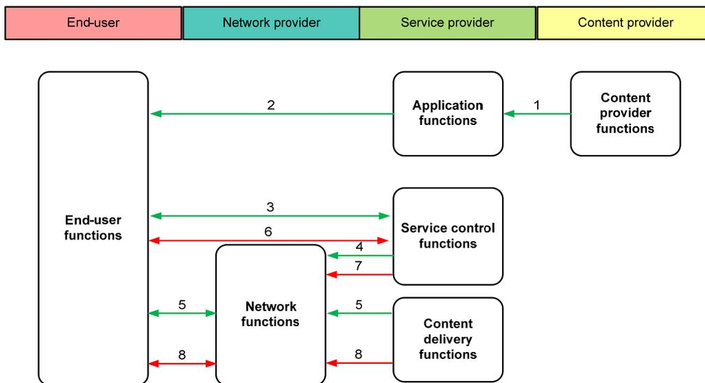
**Figure 8-8 – Use case of cooperative n-screen service with multi-terminal**
