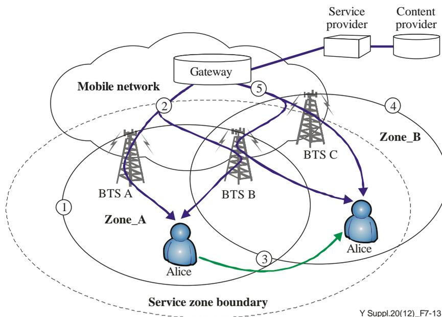
**Figure 7-13 – Mobile IPTV service based on the dynamic service zone**
