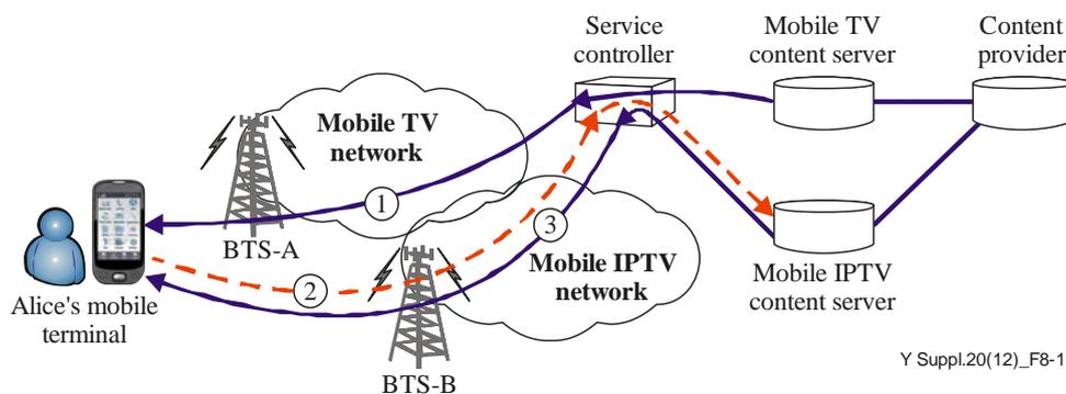
**Figure 8-15 – Cooperation scenario between mobile TV and mobile IPTV**
