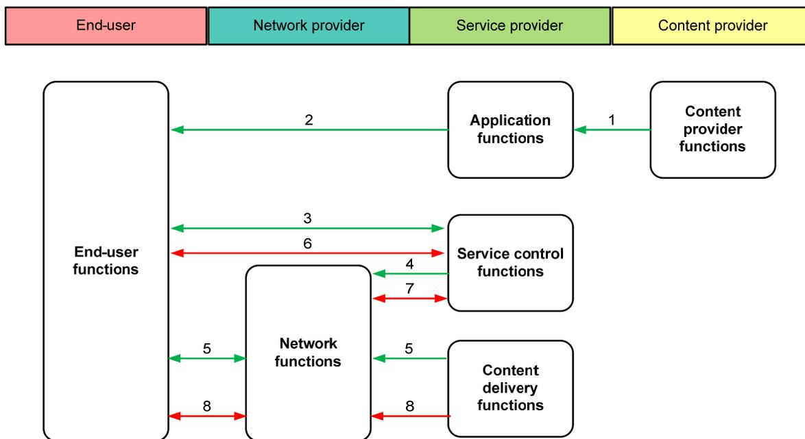
**Figure 7-6 – Use case of VoD with vertical mobility**
