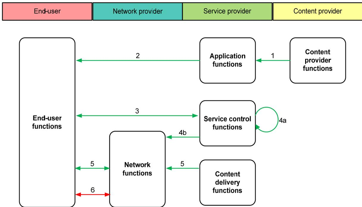
**Figure II.3 – Use case of web-based mobile IPTV**
