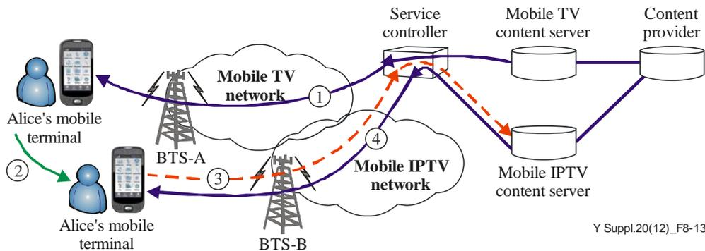
**Figure 8-13 – Service transition scenario between mobile TV and mobile IPTV**
