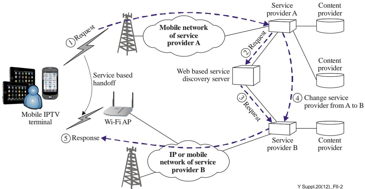
Figure II.2 – Sample scenario for web-based mobile IPTV
