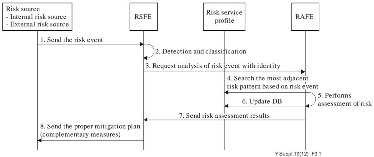
**Figure 9-1 – Information flows and actions associated with a risk analysis service procedure**
