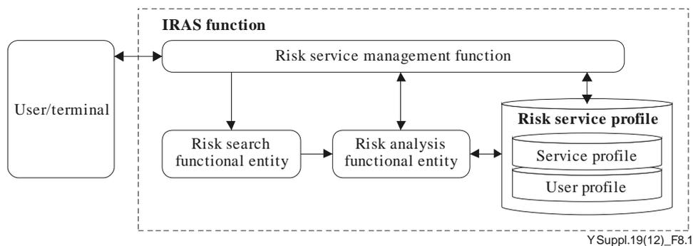
**Figure 8-1 – Functional model for an execution function when the IRAS is invoked by a user terminal**
