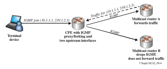
Figure 9-4 – IGMP Proxy in forking mode
