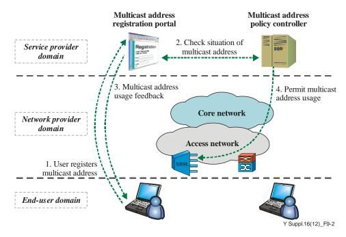
**Figure 9-2** – **Control procedure for multicast address**
