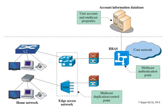
Figure 9-5 – Example of network architecture and functional components for multicast user management
