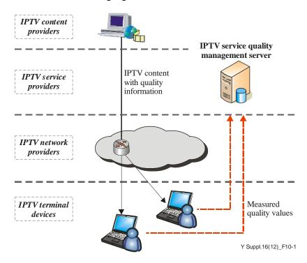
Figure 10-1 – IPTV service quality measurement using a client-server model
