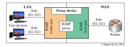
**Figure 9-3** – **Functional model of IGMP proxy**
