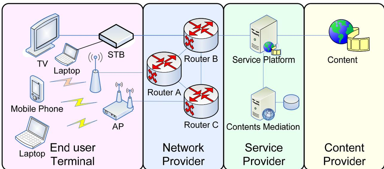
**Figure 13 – Overall configuration of IPTV over FMC**
