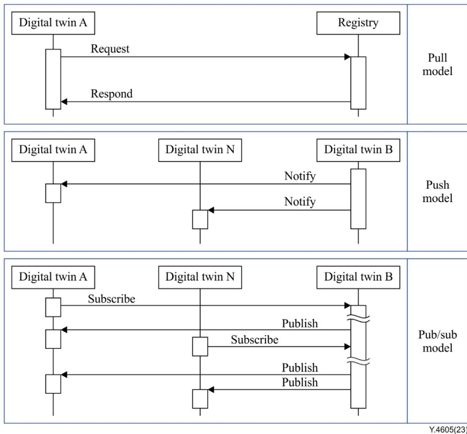
**Figure 1 – Information exchange models between the components of digital twin federation**
