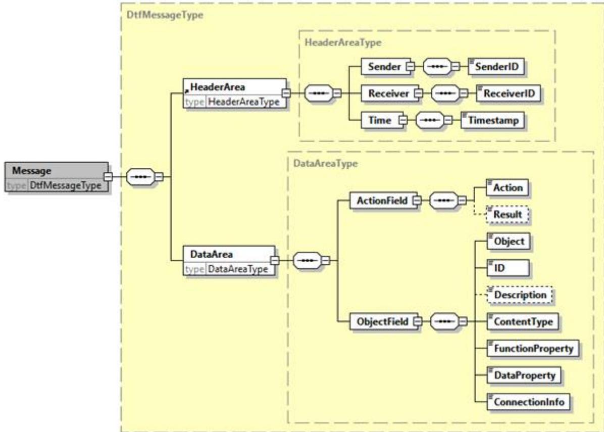
Figure II.1 – XML schema diagram of message structure
