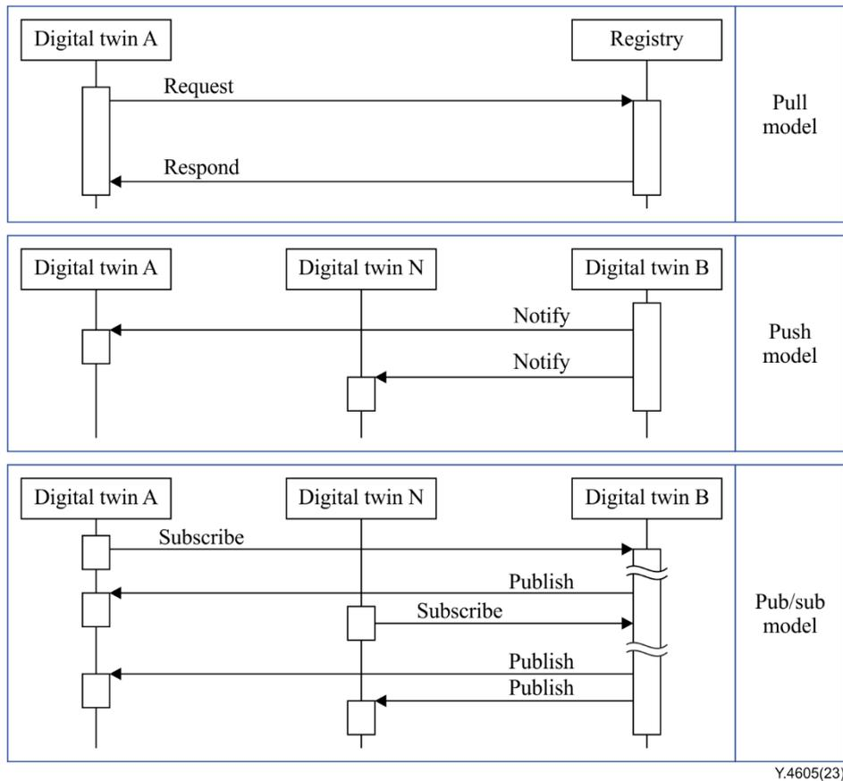
**Figure 1 – Information exchange models between the components of digital twin federation**
