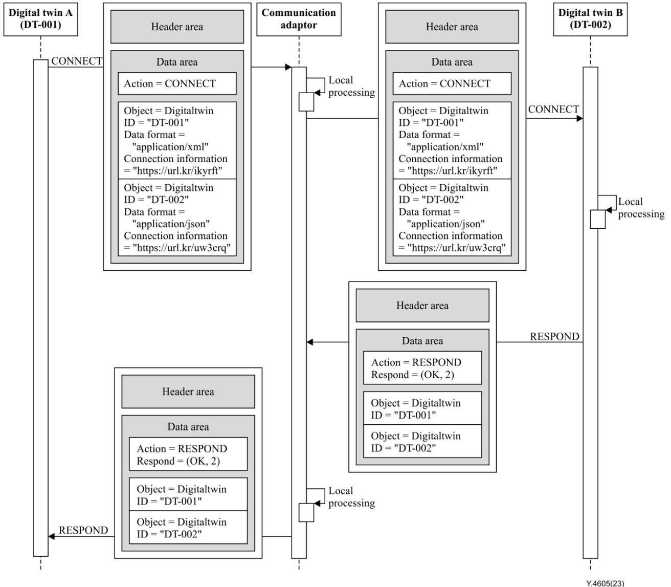
Figure I.5 – An example of indirect communication establishment
