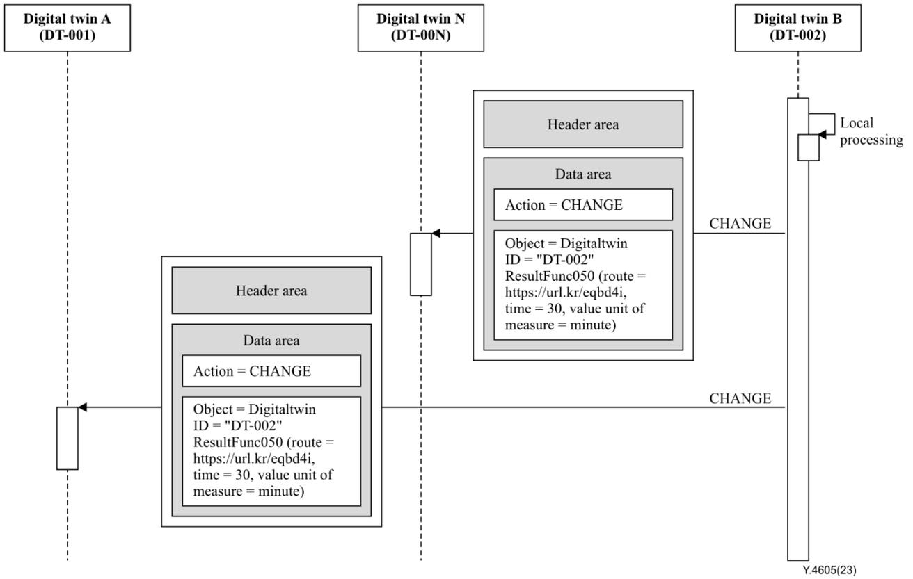
**Figure I.6 – An example of direct information exchange**
