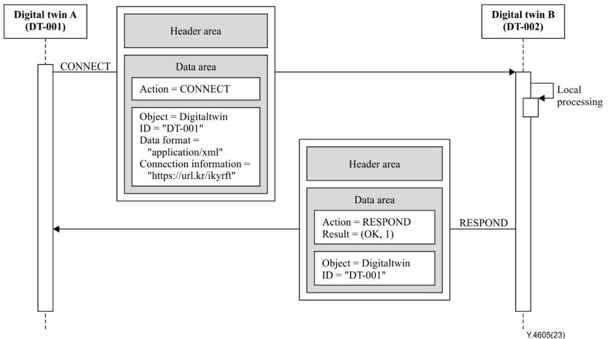
**Figure I.4 – An example of direct communication establishment**
