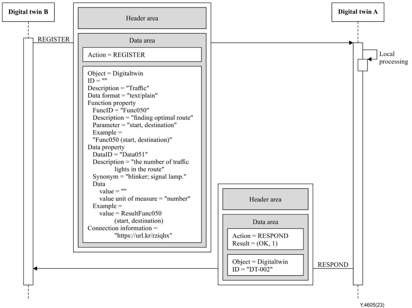
**Figure I.2 – An example of feature information registration between digital twins**
