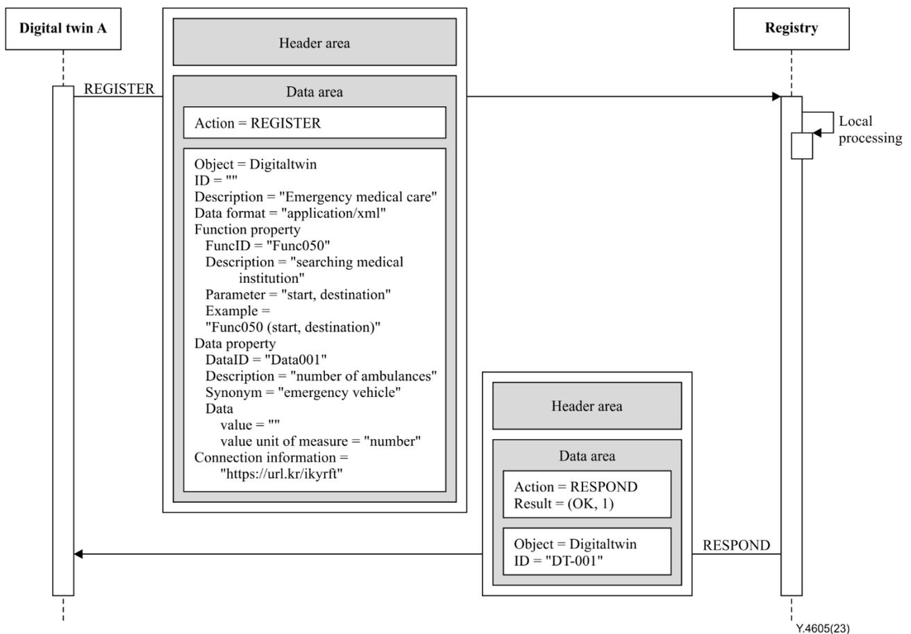
**Figure I.1 – An example of feature information registration between a digital twin and a registry**
