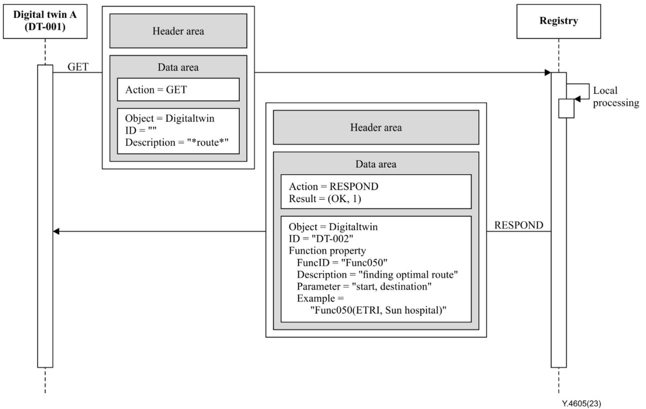
**Figure I.3 – An example of candidate digital twin discovery**
