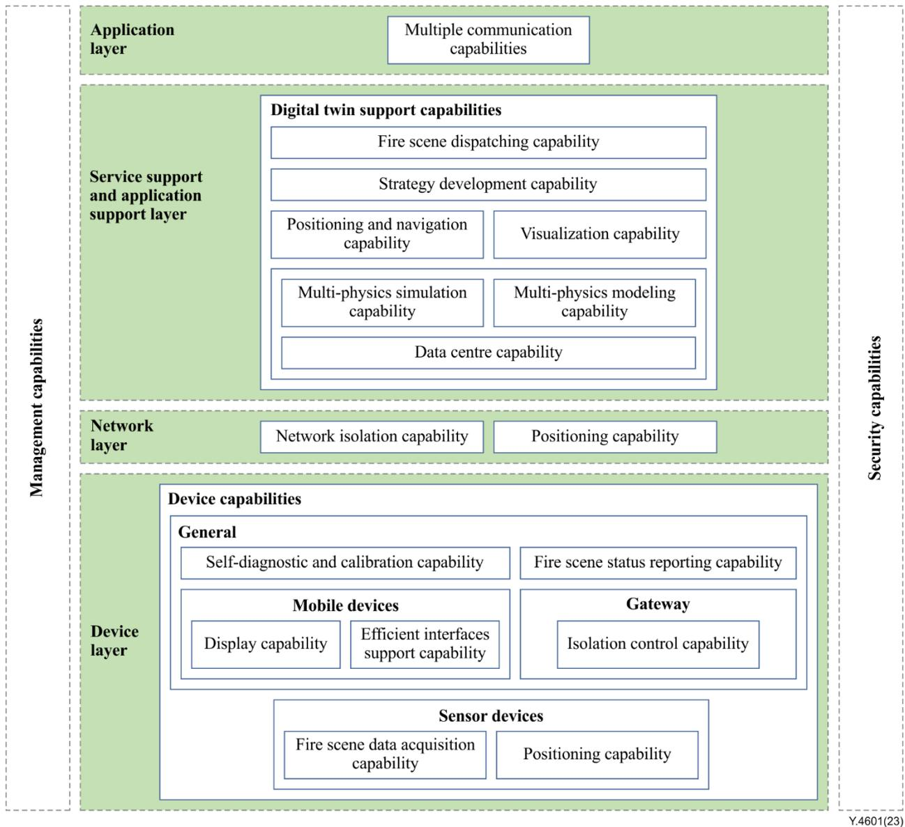
**Figure 2 – Capability framework of the smart firefighting system**
