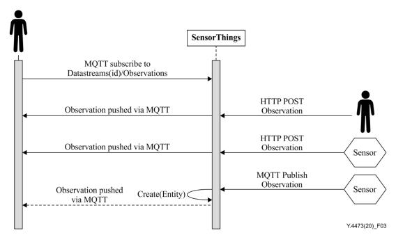
Figure 3 – Creating Observations using MQTT publish, and receive notifications for Observations with MQTT
