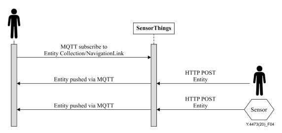
Figure 4 – Sequence diagram for receiving updates using MQTT subscribe
