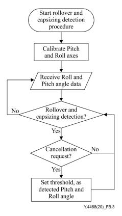
Figure B.3 – Flow of rollover or capsizing detection procedure
