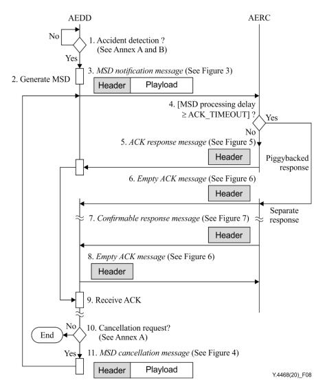
Figure 8 – Sequence of request-response operation between AEDD and AERC
