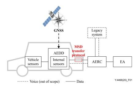
Figure 1 – Scope of MSD transfer protocol
