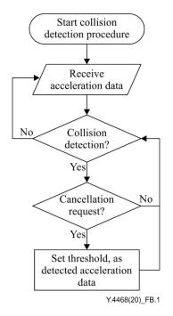
Figure B.1 – Flow of collision detection procedure
