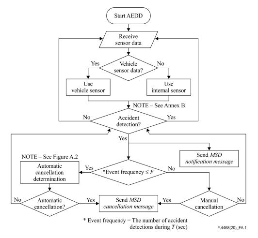
**Figure A.1 – Flow of AEDD operation procedure**
