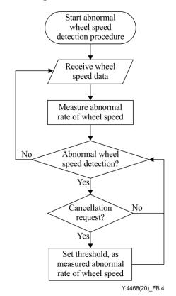
Figure B.4 – Flow of abnormal wheel speed detection procedure
