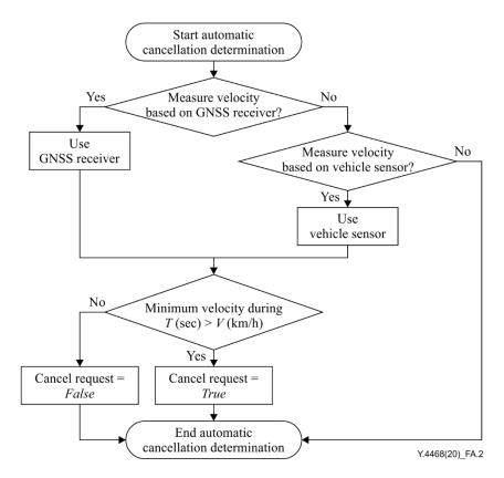
Figure A.2 – Flow of automatic cancellation determination procedure
