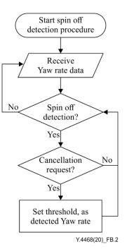
Figure B.2 – Flow of spin off detection procedure
