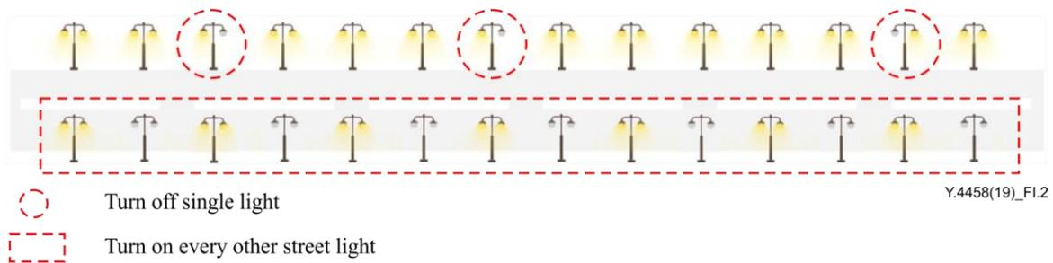
**Figure I.2 – An example of remote control of single light**
