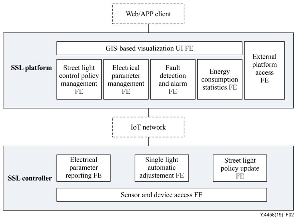
Figure 2 – Functional architecture of a smart street light service
