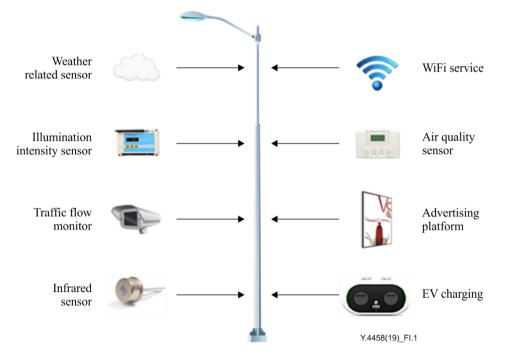
Figure I.1 – An example of a smart street light
