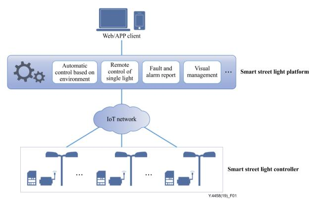
Figure 1 – Conceptual model of smart street light service systems
