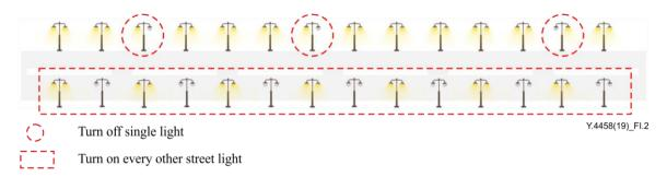
Figure I.2 – An example of remote control of single light
