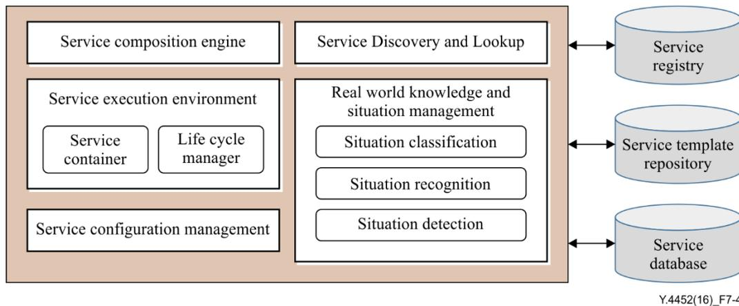
**Figure 7-4 – Functional capabilities of the service level**
