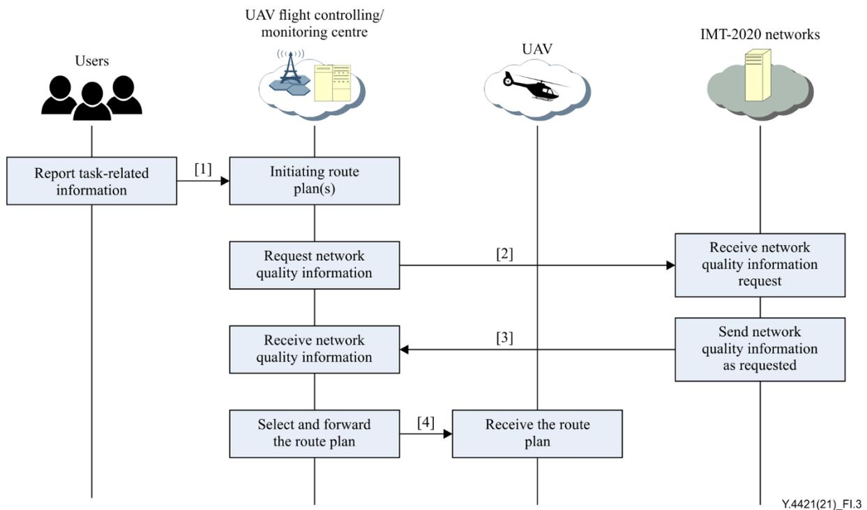
**Figure I.3 – UAV route planning based on IMT-2020 networks**
