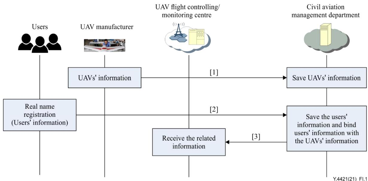
**Figure I.1 – The UAV and the user are registered based on IMT-2020 networks**
