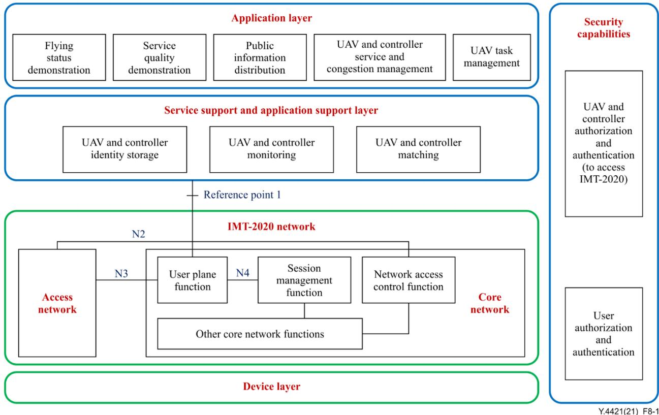
**Figure 8-1 – Functional architecture of UAVs and UAV controllers using IMT-2020 networks**
