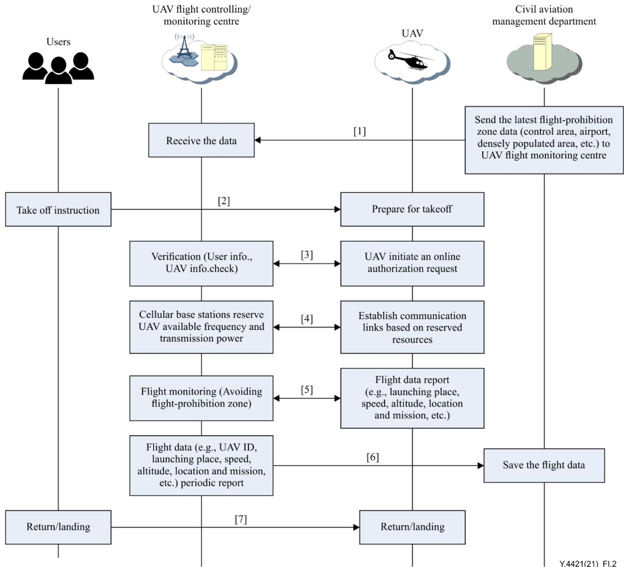
**Figure I.2 – UAV security flight monitoring process based on IMT-2020 networks**
