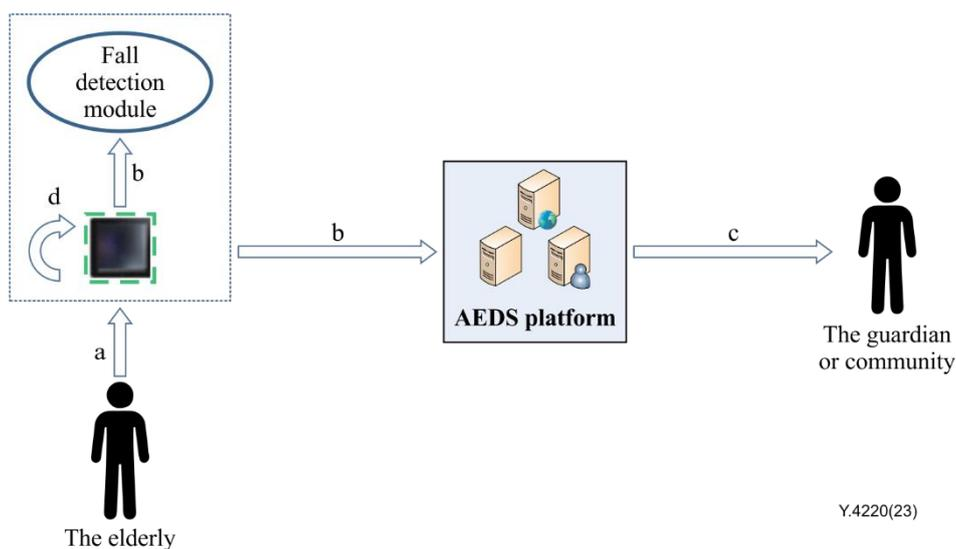
**Figure I.2 – Use case of fall monitoring for the elderly with the AEDS devices acting as a millimetre-wave radar**
