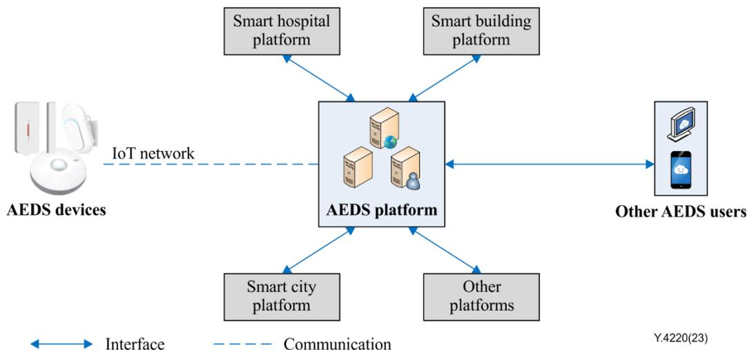
**Figure 1 – Overall conceptual diagram for abnormal event detection system for smart home**
