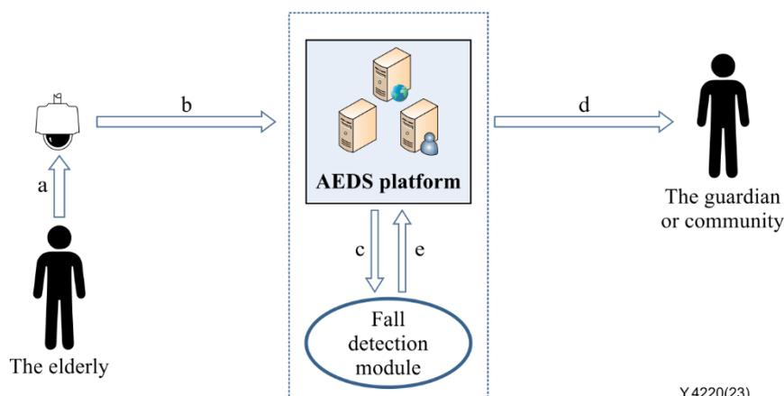
**Figure I.1 – Use case of fall monitoring for the elderly with AEDS device installed in the home acting as a camera**
