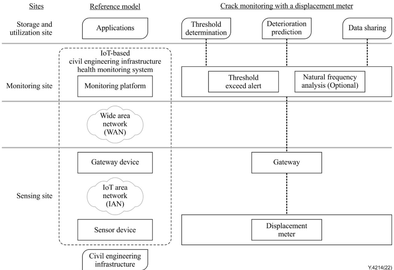
**Figure I.2 – Crack monitoring with a displacement meter**
