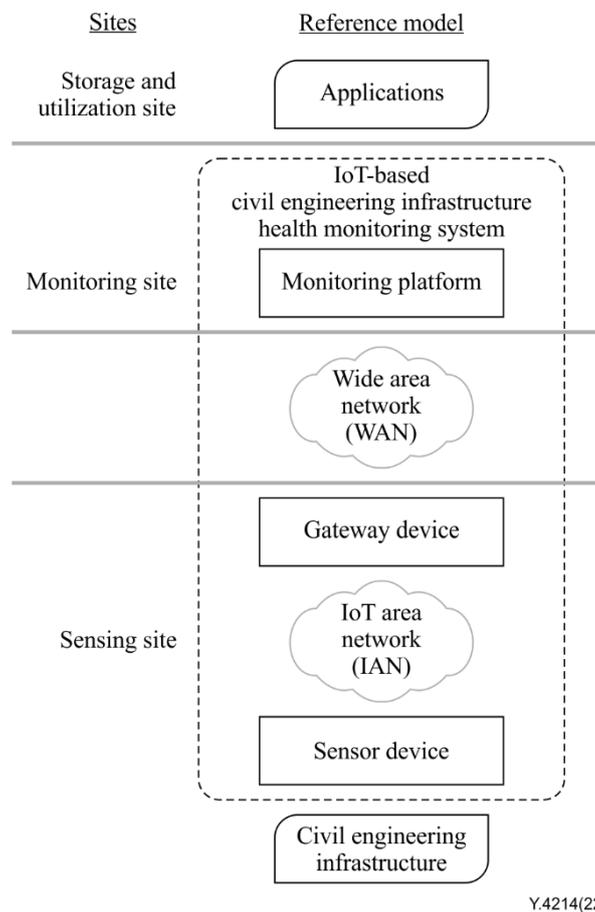
**Figure 1 – Reference model of the IoT-based civil engineering infrastructure health monitoring system and associated sites**
