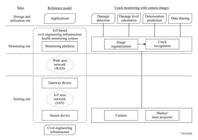
Figure I.1 – Crack monitoring with camera images
