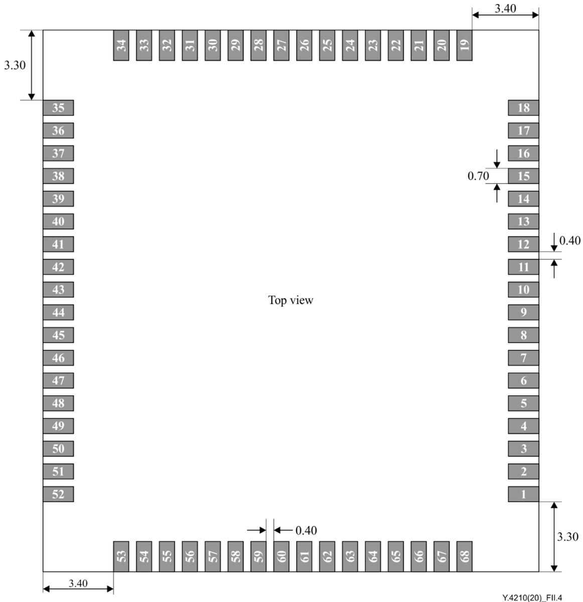
Figure II.4 – Pad size and spacing for universal communication module reference Type 4
