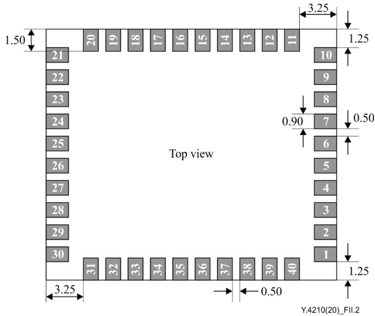
**Figure II.2 – Pad size and spacing for universal communication module reference Type 2**
