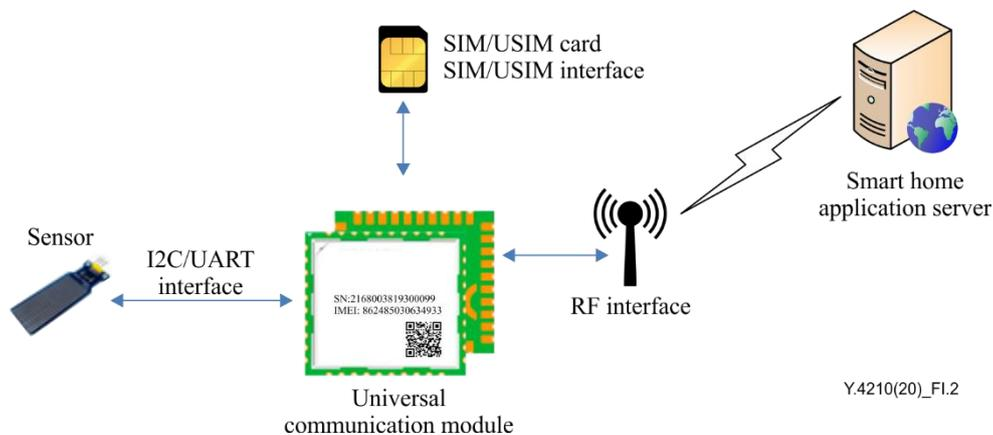
**Figure I.2 – Smart home design with universal communication module**
