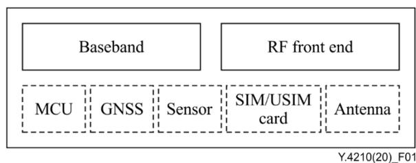
**Figure 1 – Structure of a universal communication module of mobile IoT device**
