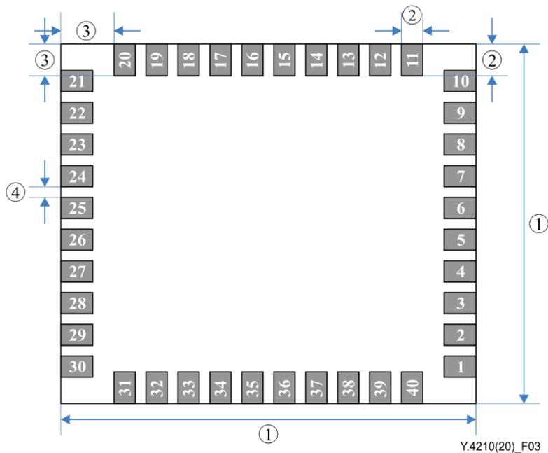
**Figure 3 – Recommended layout for small size universal communication module**
