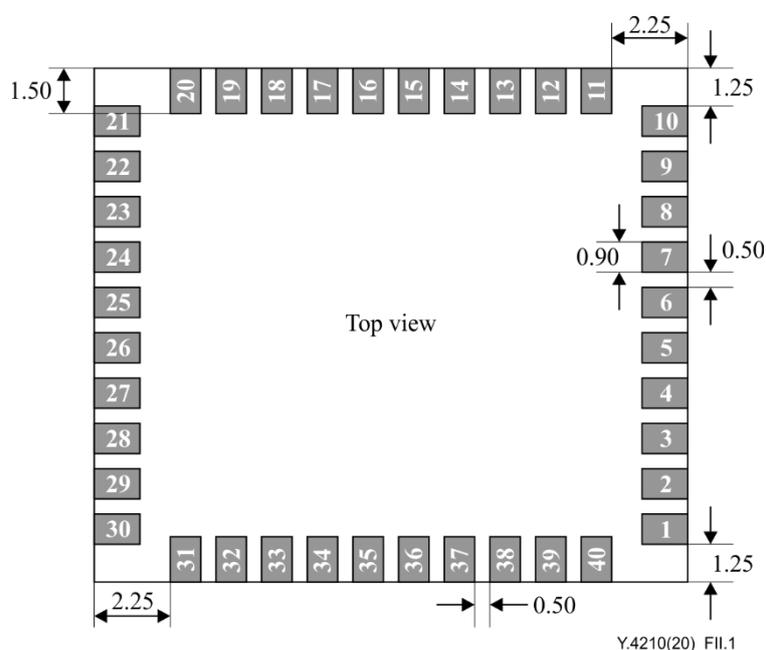
**Figure II.1 – Pad size and spacing for universal communication module reference Type 1**
