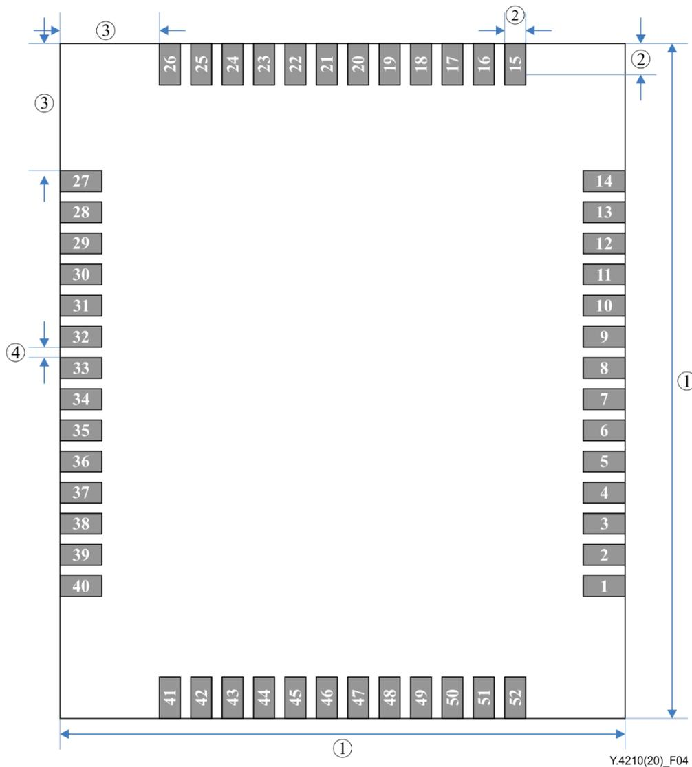
**Figure 4 – Recommended layouts for normal size universal communication module**
