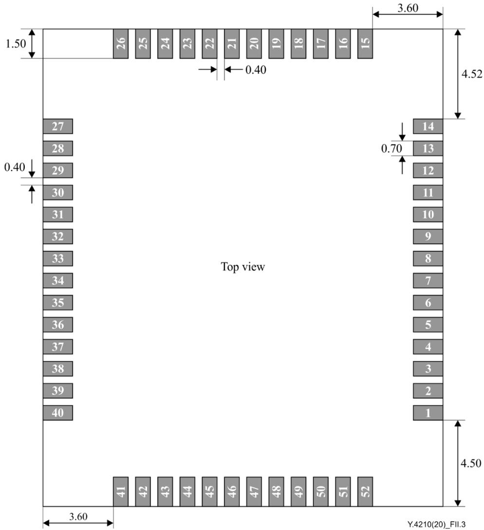
**Figure II.3 – Pad size and spacing for universal communication module reference Type 3**
