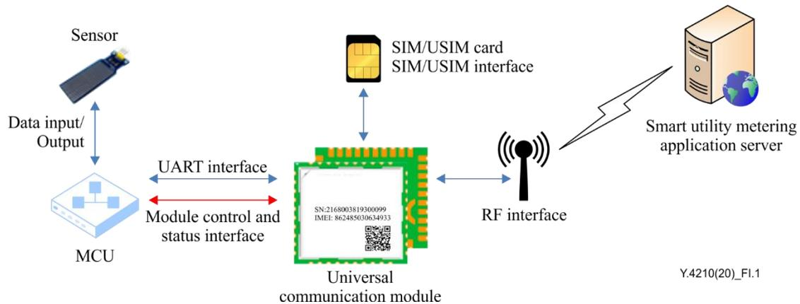
**Figure I.1 – Smart utility metering design with universal communication module**
